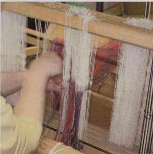
29: Threading the warp through the heddles. 30: threading warp ends through the reed.
