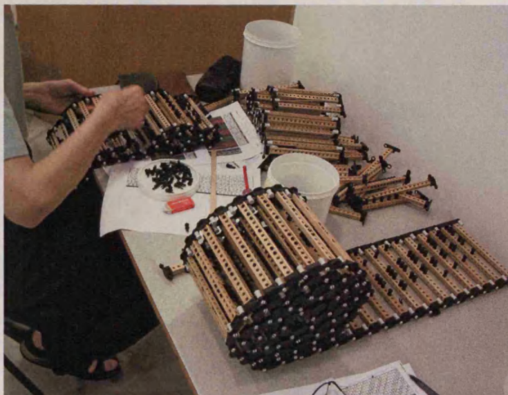
31: Preparing and pegging the lags
