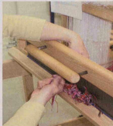
29: Threading the warp through the heddles. 30: threading warp ends through the reed.
