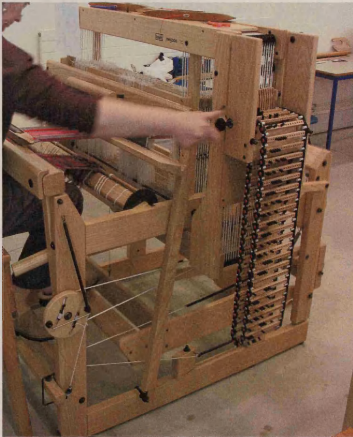
37: mastering control of a dobby loom
