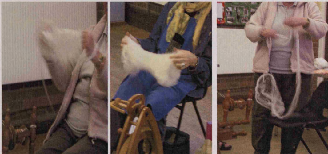
23: Pulling fibres forcibly apart 24: Aligning fibres to make a roving 25: winding the roving prior to spinning
