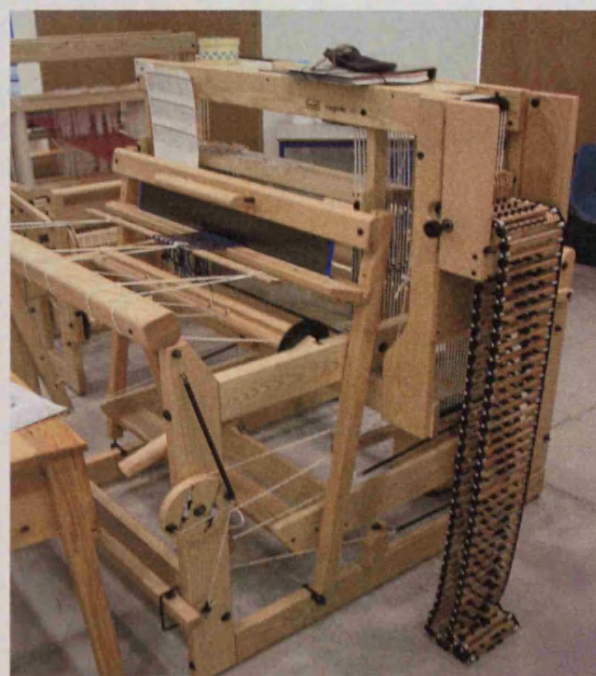
32: The chain in place on the loom
