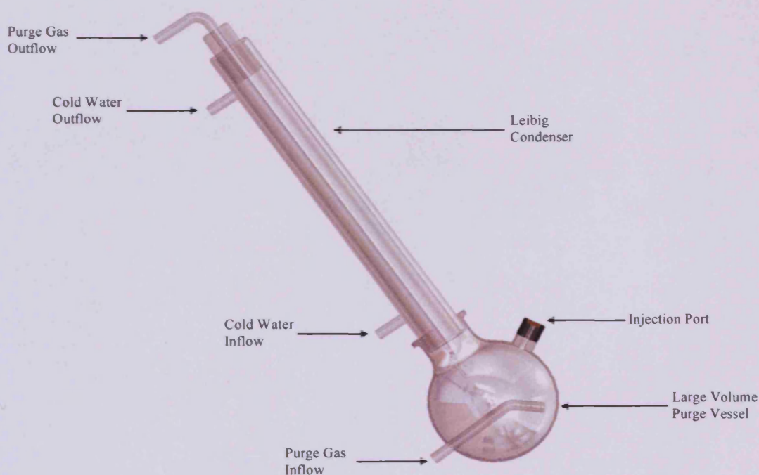
Figure 2.3. Schematic diagram of the glassware developed for refluxing vanadium III chloride reagent.
