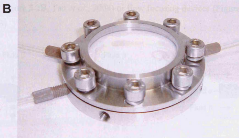
Figure 3.1: The microfluidic evaluation platform (MicroPlant™) used in all microfluidic experiments. A) Expanded schematic showing the components of the microfluidic evaluation rig. B) Photograph showing evaluation device sealed, with a microfluidic chip inserted and fluid connectors
