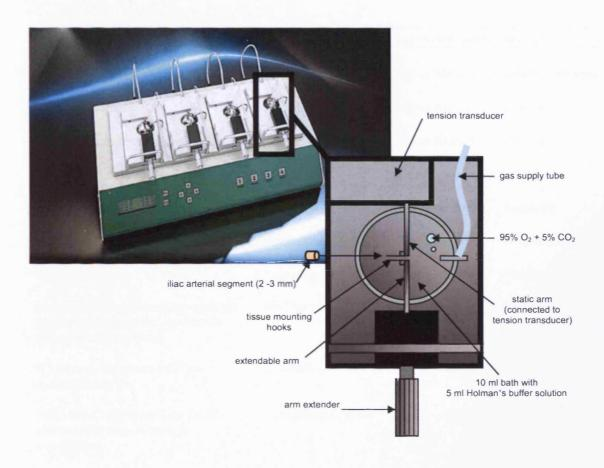
**Figure 2.2** Schematic of a single channel of the Mulvany Myograph (original diagram). Photograph obtained from Danish Myotechnology, Aarhus, Denmark.
