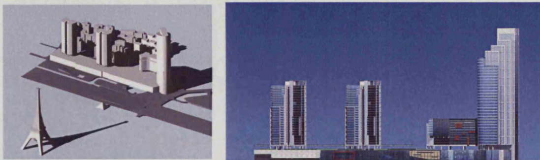
Casefigure 7.4 The 'extreme' design, which was the only massing option to meet the sunlight regulation and the maximum floor space.
