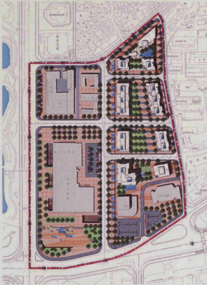
Casefigure 9.2 The masterplan by CAUPD in 2003 (Source: China Academy of Urban Planning & Design 2005). Six urban blocks were formed providing a permeable environment. The site for the Grand Theatre seemed to have over-generous building setbacks and provided a large urban plaza in its front. The site for the two important banks were enlarged to allow additional office space to be built for financial sectors, but the existing ground floor car park for the south-east site was retained, providing an unpleasant environment. The three residential blocks to the north mixed with commercial uses were building to the site edges, with a central green in the middle.
