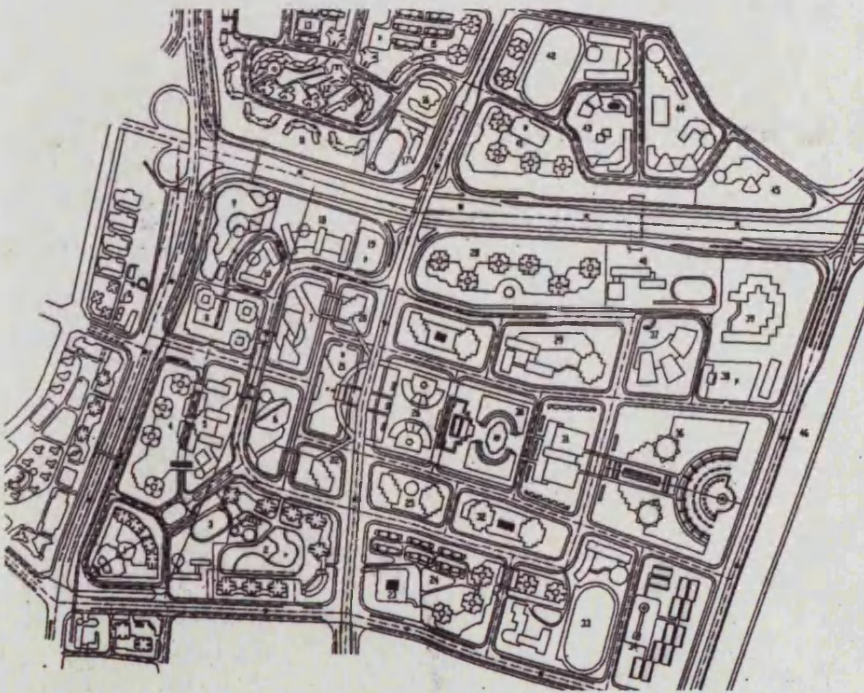
Masterplanfigure 3.2 The first detailed plan for the NSCD featured wide buildings standing alone in the middle of every urban plot. The idea of creating a district centre with a strong east-west commercial axis remains in the latter plans.
