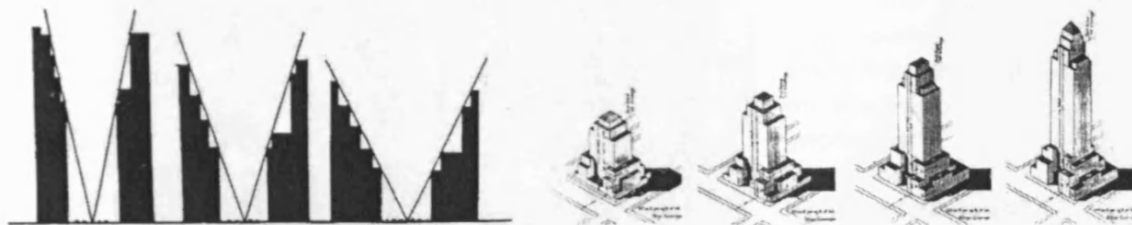
Fig. 2.2.4 Zoning's building setback requirement in New York. Left: building setbacks prescribed by the zoning ordinance of 1916; Right: 'setback style' generated by this ordinance (Source: Loukaitou-Sideris and Banerjee 1998 pp.49-51).
