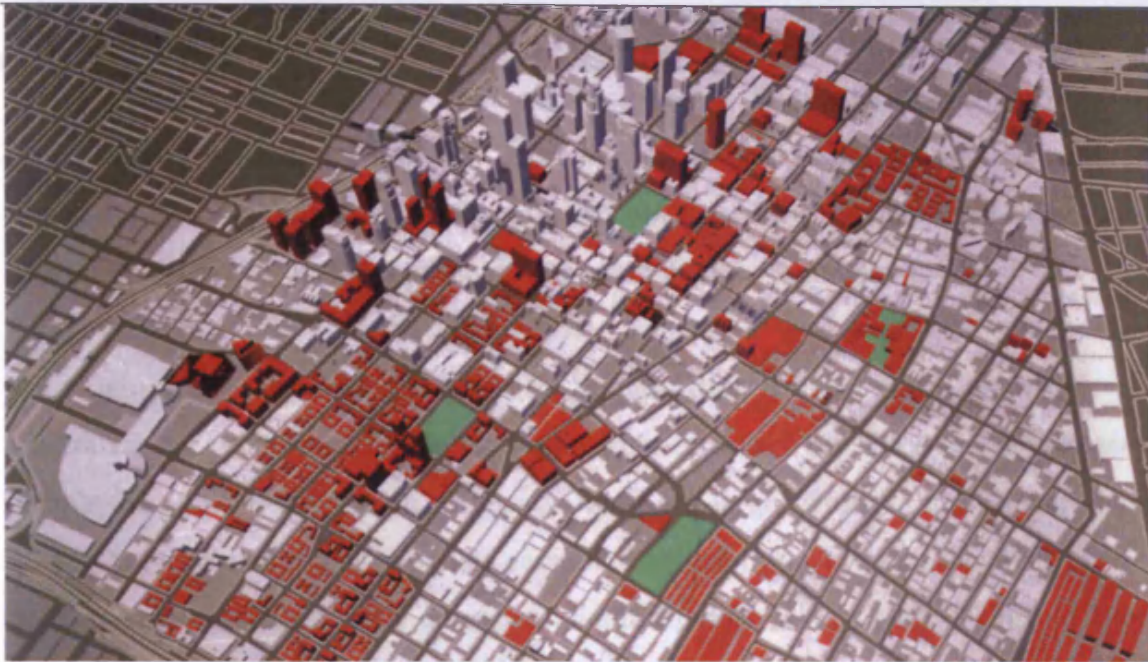
Fig. 2.2.9 Section of the 2020 Los Angeles Downtown Plan (Source: Katz 1994), addresses the extensive physical changes (in red) and the social and economic ones, guiding the incremental downtown development. A development code is provided to replace the existing zoning code.
