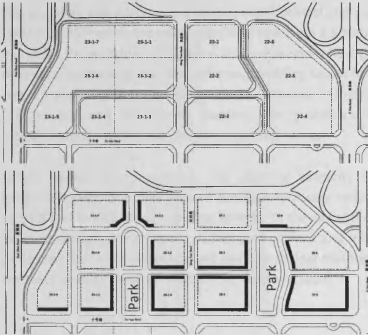
Masterplanfigure 2.3 Top: the original land parcelization of the block. Bottom: Urban design guideline for Block 22 & 23-1 by SOM in 1998 (Adapted from Li 2002). The way it deals with land subdivision, public space and street wall has had a fundamental impact on Shenzhen's urban design discourse.
