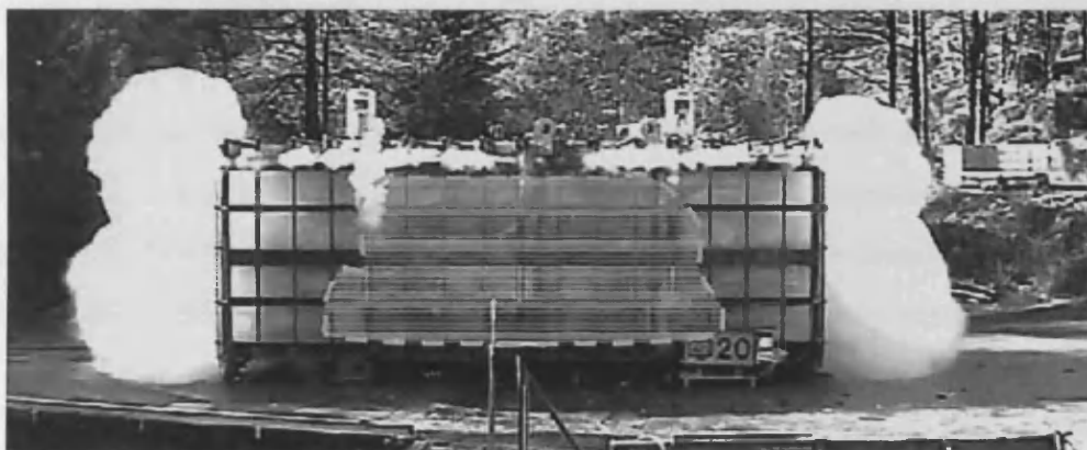
Figure 8.32 Photograph showing the maximum extent of flame through water mist barrier generated by Micromist atomisers
