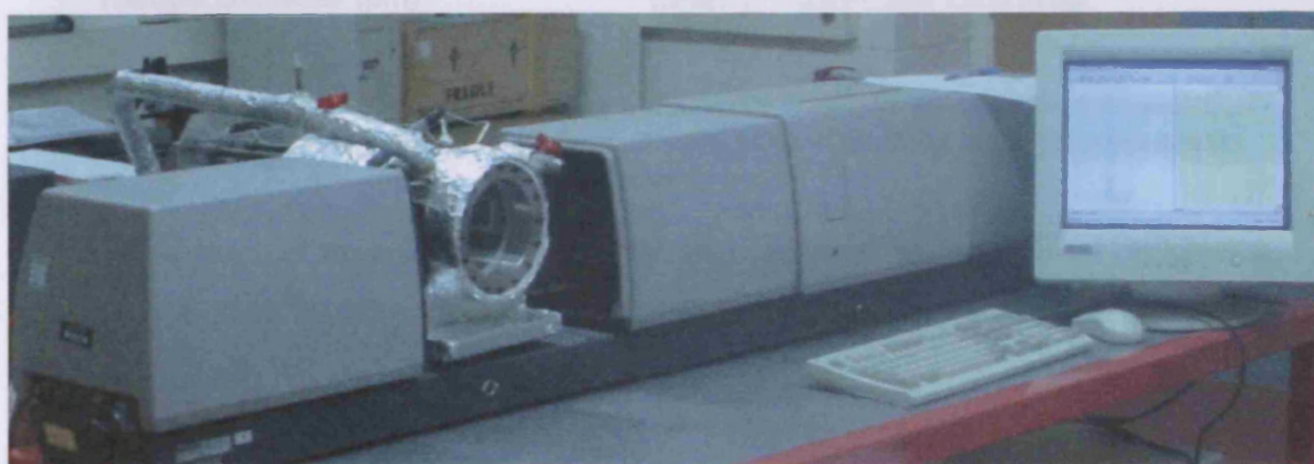
Figure 4.7 Photograph of Cardiff cloud chamber in Malvern Mastersizer
