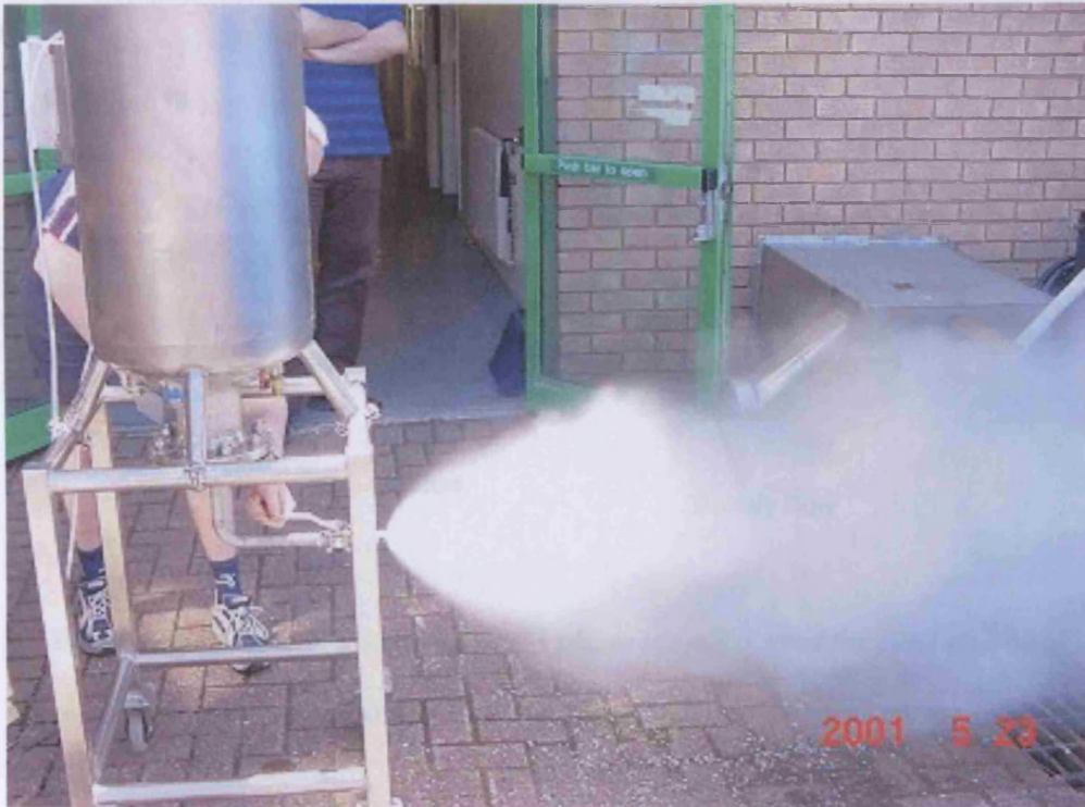
Figure 8.5 Flashing release from Micromist atomiser
