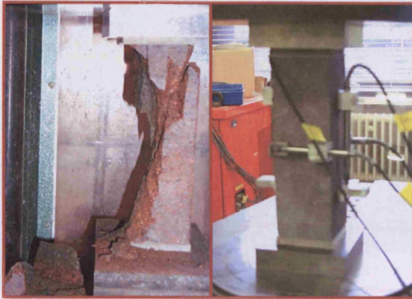
Plate 3-3: Stress strain relationship brick test
