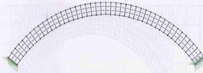
Figure 7-10: Shallow arch barrel non-linear model
