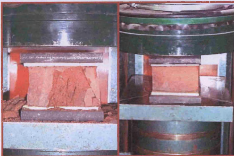
Plate 3-2: Compression bricks test
