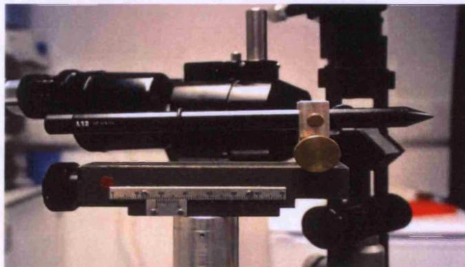
**Fig 3.3:** The Cochet-Bonnet Aesthesiometer attached to a slit-lamp holder.
