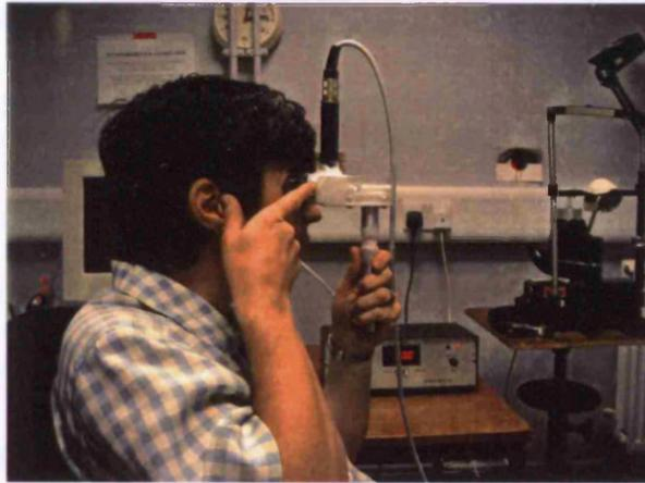
**Fig 3.12:** The swimming goggle of the evaporimeter attached to the eye for the measurement of the tear film evaporation from the ocular surface.
