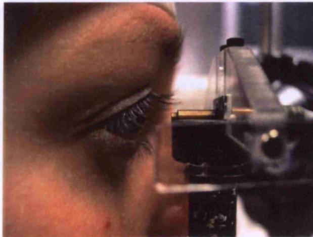
**Fig 3.2:** Positioning the stimulus air-jet close to the eye.
