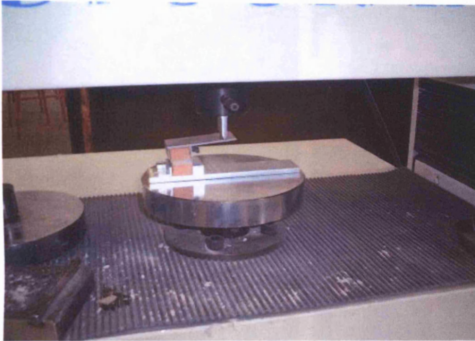
D 3.1. The bond wrench test system for one-sixth scale couplets
