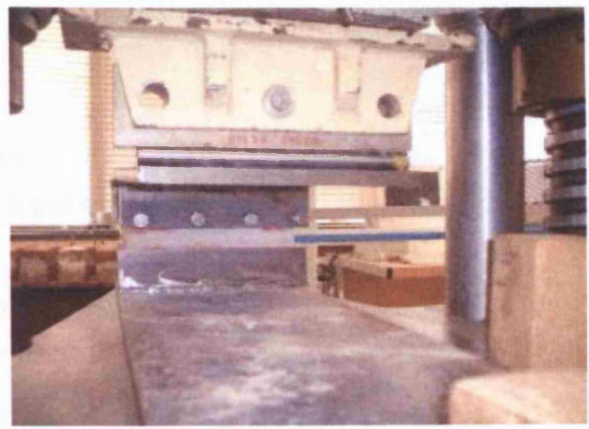
D 4.4 The mechanism for loading the full scale bond wrench testing jig.
