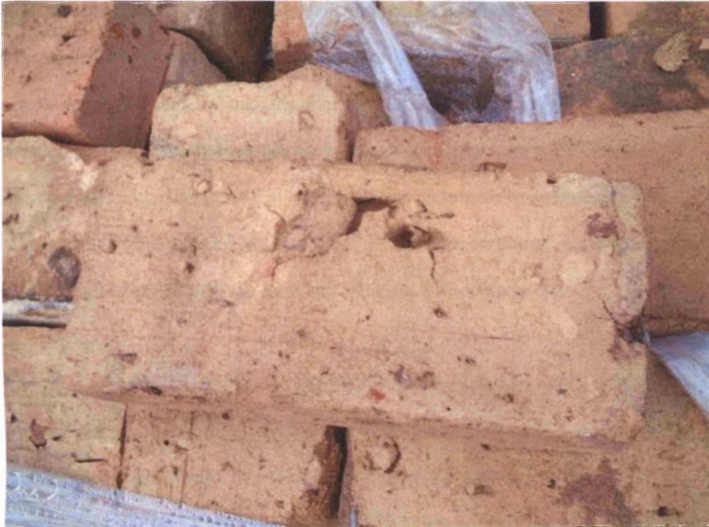
Figure 2-11. Wire cut brick containing foreign material
