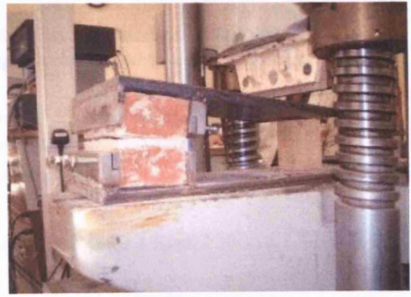
D 4.6. The full-scale bond wrench test after failure has occurred
