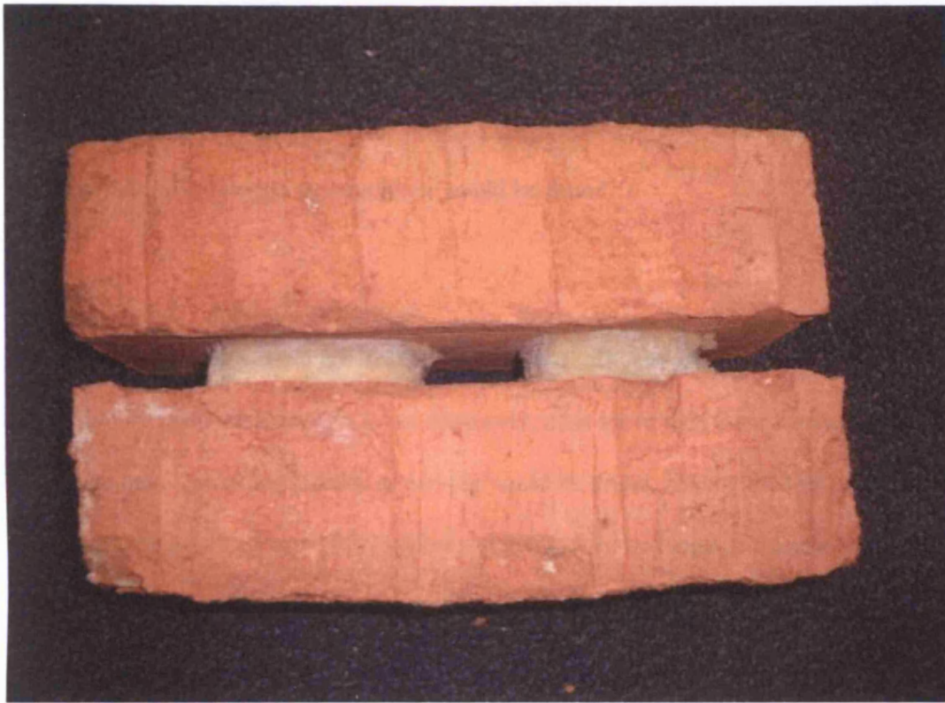
Figure 6-13. The couplet with a reduced mortar area
