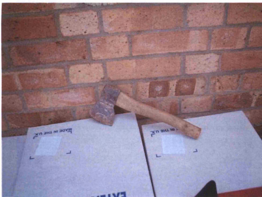
Figure 2-9. Typical hand-axe used to clean lime mortar from bricks
