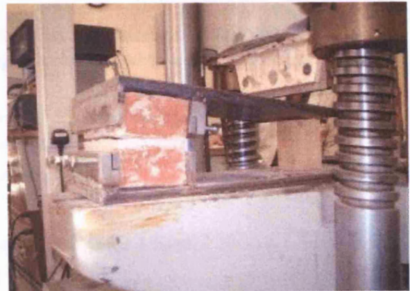
D 4.6. The full-scale bond wrench test after failure has occurred
