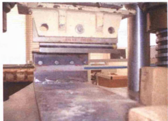
D 4.4 The mechanism for loading the full scale bond wrench testing jig.
