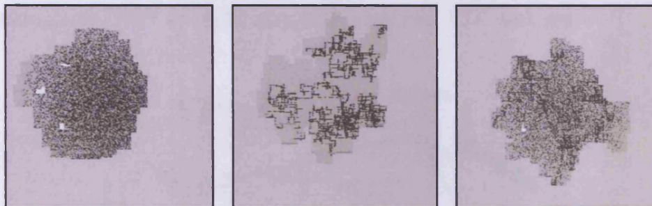
Figure 6.4: SE1 (left) models a town where traffic is distributed as a function of distance from the centre. SE2 (middle) models a town with street-style traffic distribution. SE3 (right) combines SE1 and SE2. RTP are light gray, STP gray, and TTP dark gray
