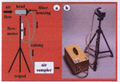
Figure 3.2: The monitoring equipment used for the collection of PM<sub>10</sub>.
