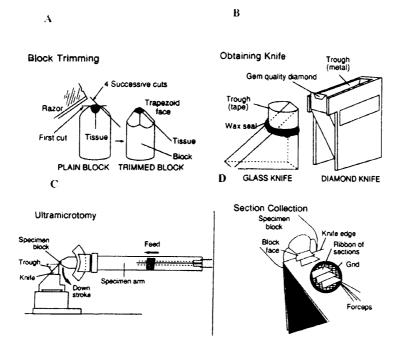
Figure 2.7. The four steps involved in ultramicrotomy process are (A) cutting the resin block using a razor blade to expose the underlying tissue and to form a trapezoid cutting face, (B) making glass knives with which to cut ultrathin sections, (C) placing the trimmed block in the ultramicrotome, and (D) cutting the ultrathin sections using a knife edge followed by picking up the floating sections with a copper grid (from Bozzola and Russell, 1992).
