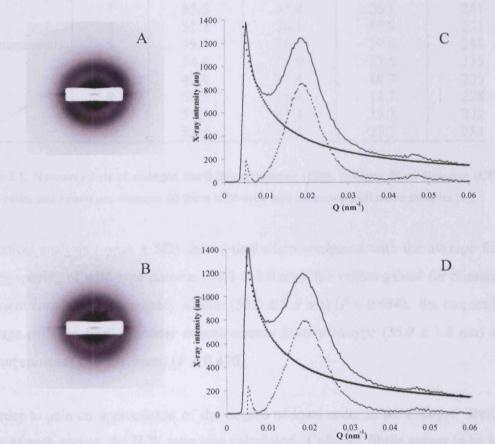
Figure 5.2. XRD patterns of wild-type (specimen 4 in Table 1) (A) and mimecan-deficient (specimen 12 in Table 1) (B) mouse corneas with similarly well-defined 1<sup>st</sup> order equatorial reflections, indicative of well-ordered corneal stromal collagen fibrils. C and D are the respective X-ray intensity profiles (solid lines), from which the fitting and subtraction of a power-law background function (squares) produces the resultant XRD pattern measured (dotted lines).
