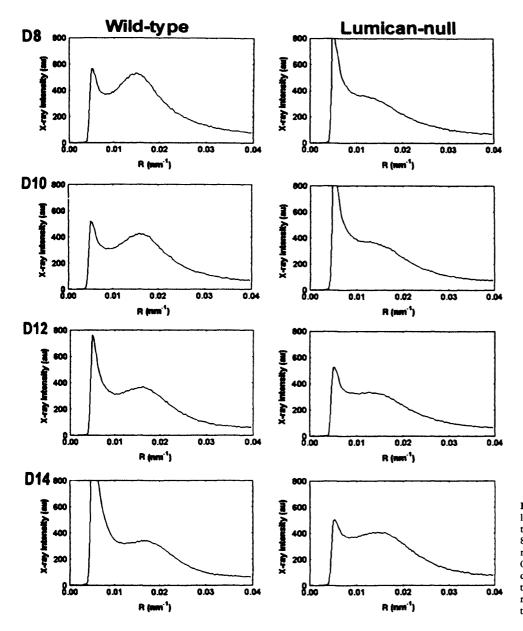
FIGURE 1. X-ray intensity scans across low-angle synchrotron x-ray diffraction patterns from the corneas of day 8 (D8) to 14 wild-type and lumicannull mice. The peak in the region of 0.013 to 0.018 nm<sup>-1</sup> represents the collagen interfibrillar x-ray reflection that arises from the regularly arranged collagen fibrils that constitute the stromal extracellular matrix.
