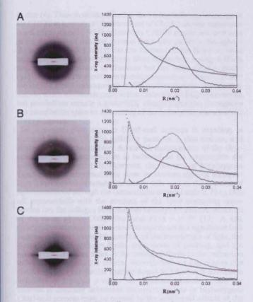
Fig. 6. Synchrotron x-ray fiber diffraction patterns from the corneas of WT (A), heterozygous (B), and homozygous (C) Chst5-null mice revealing a more diffuse collagen interfibrillar x-ray reflection in the homozygous situation. Background-subtracted peaks in the x-ray intensity profiles from the patterns confirm the diffuseness of the interfibrillar reflection and enable calculation of the mean center-to-center collagen interfibrillar Bragg spacing.
