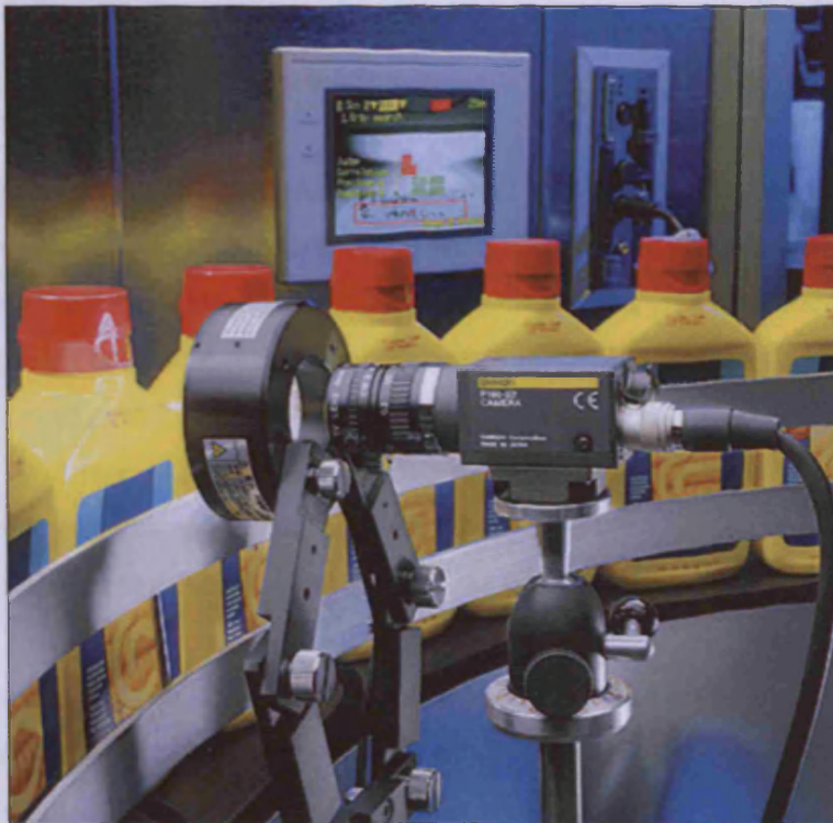
Figure 5. A sample machine vision quality testing of chemical bottles system, image used with the kind permission of Omron Electronics LLC.
