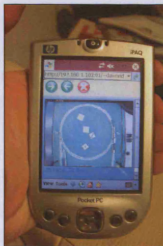
Figure 86. Train control being performed via a web browser on a Compaq iPaq PDA. Note that the interface has been slightly simplified, and the browser has automatically resized the image to fit the smaller screen. Alternative camera names are placed as text beneath the image.
