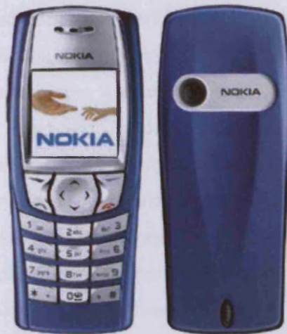
Figure 103. Nokia 6610i mobile phone, front and back (note camera lens to the left of the Nokia logo on the back)
