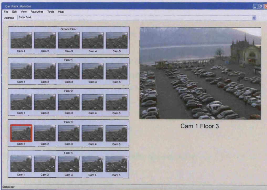
Figure 96. Car park monitoring GUI mock-up, showing 25 camera image thumbnails and selectable full-resolution display of camera images
