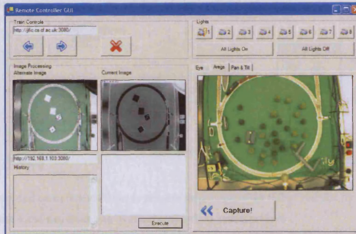
Figure 87. Combined interface for remote image processing, train control and lighting. Connected to 1x IPE, 2xEC and 3xNACs, merged into the same interface
