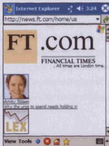
Figure 83. Simplification of a web page by Pocket Internet Explorer, displaying automatic image resizing to adapt to the form factor of the PDA device
