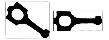
Figure 1. Representing an arbitrary 2D shape by the minimum-area rectangle. Left: rotation is prohibited. Right: rotation is permitted. The object has been rotated so that the axis of minimum second moment ("principal axis") is horizontal. Orienting all of the shapes like this often results in a more efficient packing.
