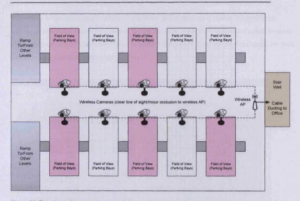
Figure 95. Top-down diagram of a car park floor with multiple WNACs, their fields of view and line of sight to a wireless access point
