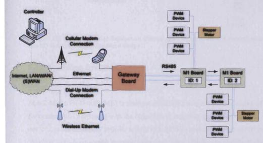
Figure 119 : Use of the 'Gateway' logic board to provide a network bridge for command sequences
