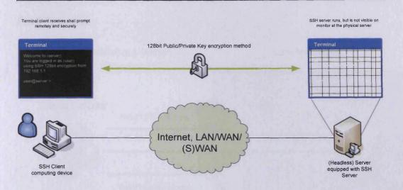
Figure 126 : SSH using encrypted traffic to 'remote' a shell session from a server to a connected client with certificate-based encryption techniques
