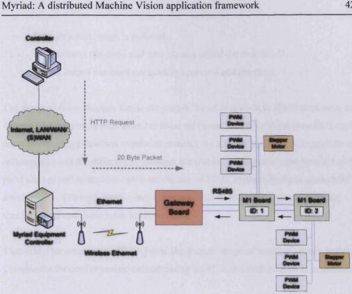
Figure 120 : Using a Myriad Equipment Control (EC) server to act as a networked interface to M1 systems, simplifying client design
