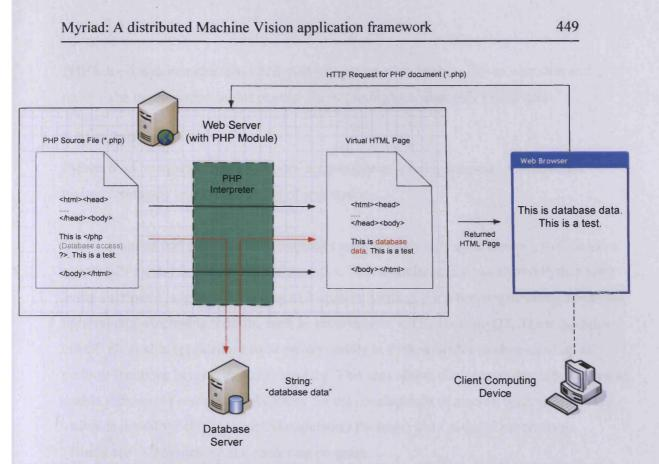
Figure 128 : Web serving dynamic data using PHP and database access, evaluating hybrid HTML-PHP script files
