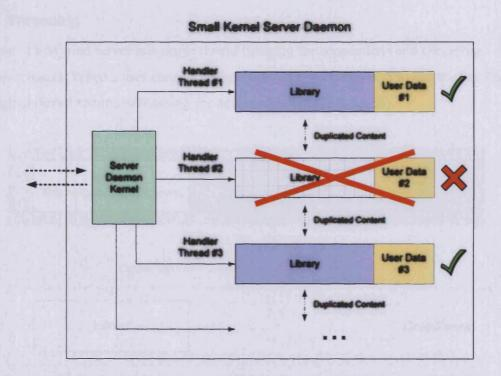
Figure 54. A small-kernel maintains separation of all client-handler code. If one client handler thread produces an error and fails, other clients are unaffected
