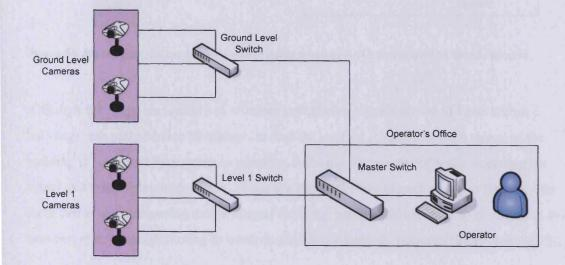
Figure 93. Monitoring the car park structure using Network Attached Cameras with multiplexing provided by conventional network switches and a single computer displaying camera images in a 'many-up' visualisation
