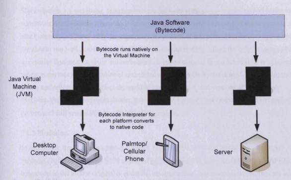
Figure 117 : Uniform Java 'byte-code' being executed uniformly across multiple computing form factors and devices through intermediary operation on a Virtual Machine
