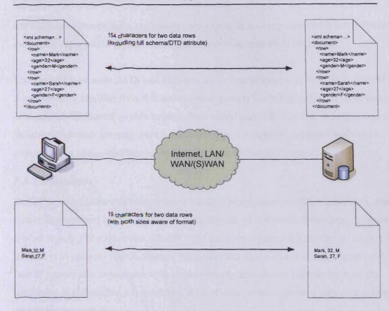
Figure 124 : Comparison of meta-data overhead for simple data tasks from XML and pure data formats
