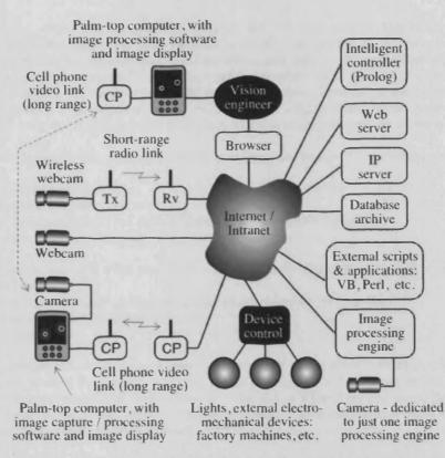
Figure 1 Distributed vision systems. Notice that cameras may be connected by cable, short-range radio, or cell-phone. Each of the modules shown here may be replicated many times, to create a complex mesh of inter-operating sub-systems.
