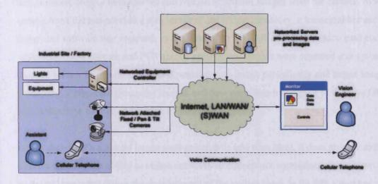
Figure 88. The intended complete solution to remote inspection of an industrial site by a Vision Engineer, with the aid of a site-local assistant and Myriad networked vision servers
