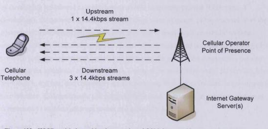
Figure 122 : HSCD multi-channel implementation of GSM data provides greater bandwidth in a multiplexed manner
