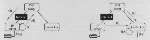
Figure 4. Operation of the Myriad-LinPacker system. Data transfers, indicated by labels (a)-(h), are defined in the text. Left: controlling the IP server, capturing an image, fitting the minimum-area rectangle around each of the blobs and saving the data. Right: Controlling LinPacker to gather the packing data, process it and output the resulting packing solution to the user.
