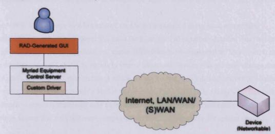
Figure 18 : Myriad control of a networked device using a custom-written device driver incorporated into a standard control server
