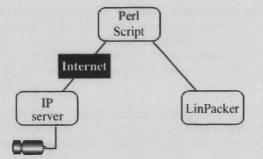
Figure 3. Myriad-LiPacker system. Both sub-systems are controlled by a Perl script, while the camera is controlled by the IP server.
