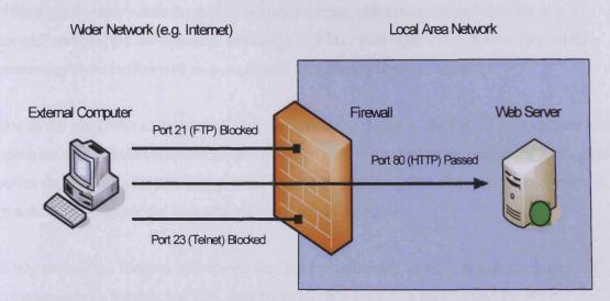
Figure 127 : Simple port-blocking method of firewalling for a server (either utilising a software firewall or hardware device)
