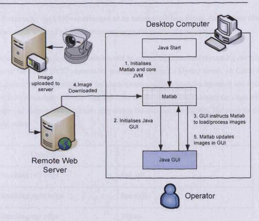
Figure 89. Matlab and Java used together to provide an image processing engine and GUI for use with networked image providers
