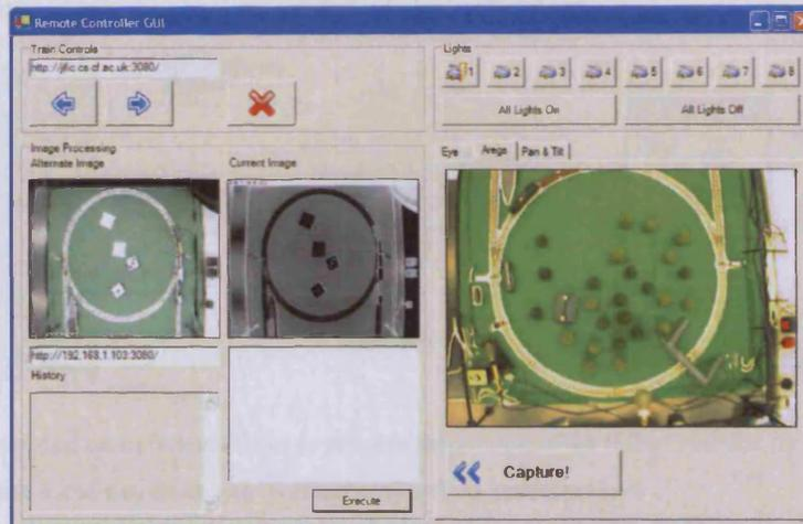
**Figure 87.** Combined interface for remote image processing, train control and lighting. Connected to 1x IPE, 2xEC and 3xNACs, merged into the same interface
