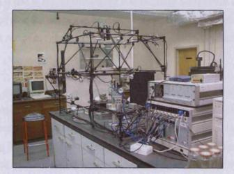
Figure 78. Photograph of the Flexible Inspection Cell prior to installation of the train set, clearly showing mounted cameras and light bulbs for variable viewpoint and lighting, control being provided by the MMB control box on the right hand side of the image
