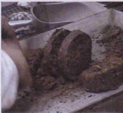
Plate 4.2. Rigidity of oil mixed soils
