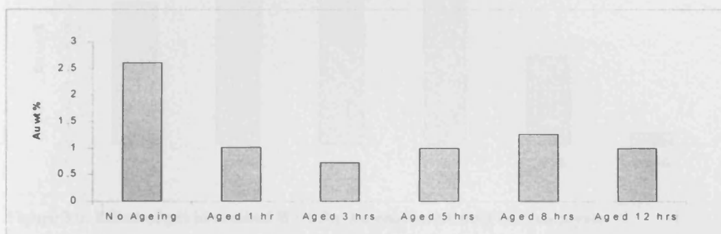
Figure 3.3. Effect of ageing at pH 8 on Au content of Au/ZnO catalysts prepared by coprecipitation at variable pH (method A)
