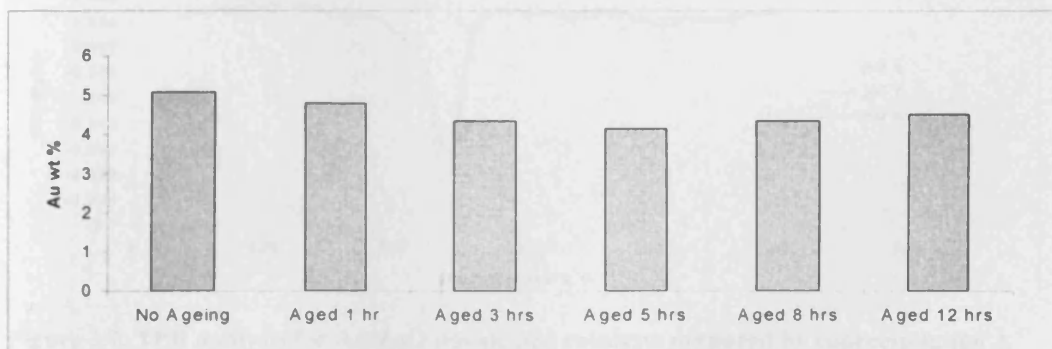
Figure 3.5. Effect of ageing at pH 6 on Au content of Au/ZnO catalysts prepared by (method B)
