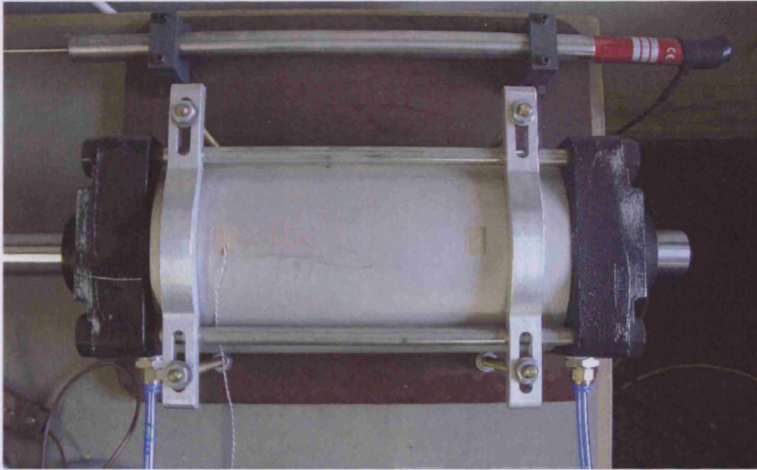
Figure 3.12: LVDT ACT 3000C mounted at the side of the pneumatic cylinder
