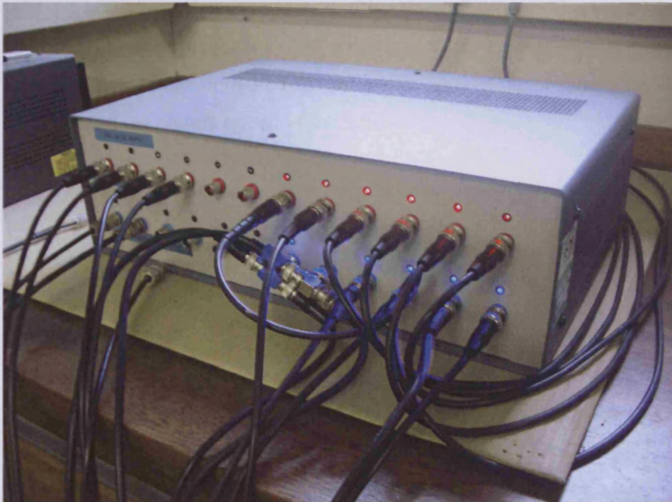
Figure 3.9(b): Voltage relay unit
