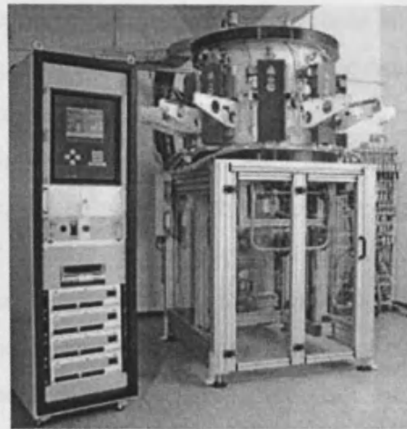
Figure 5.1: Photograph of the type of magnetron sputtering system used for Me-DLC coating tested in the experimental programme (from Balzers).
