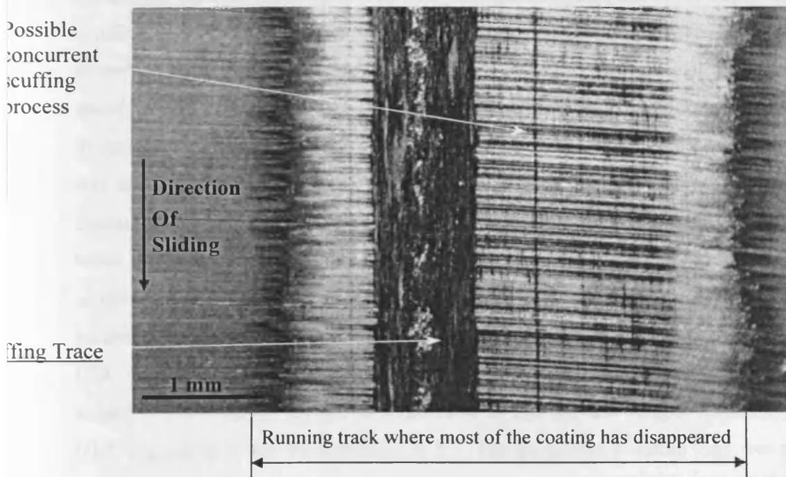
Figure 5.8: Scuffing pattern of a Case Carburised disc with Me-DLC coating sample where scuffing occurred at the edge of the track. Most of the coating has disappeared from the running track; a concurrent scuffing degradation appears to be starting in the middle of the track where the surface was in a near “superfinished” condition.
