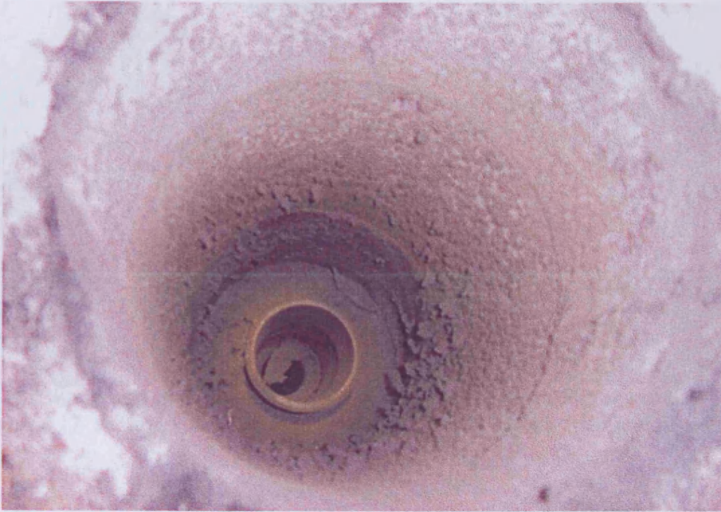
Figure 6.10 Primary reactor deposition from pure coal firing
