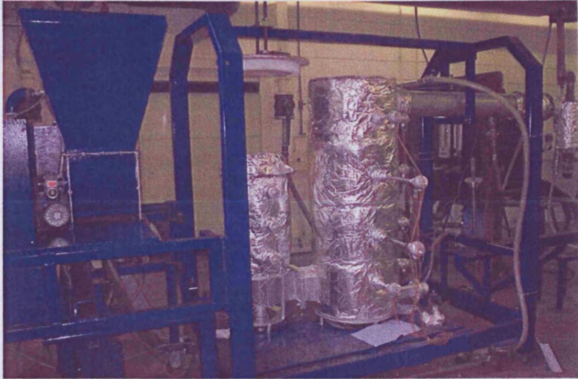
Two-stage combustor assembly on the frame bench
