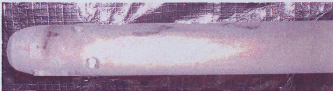
Figure 5.5 Deposit collected on the original deposition probe when firing CSF000
