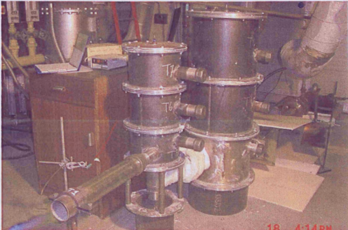
Figure 3.4 The two-stage combustor during refractory curing
