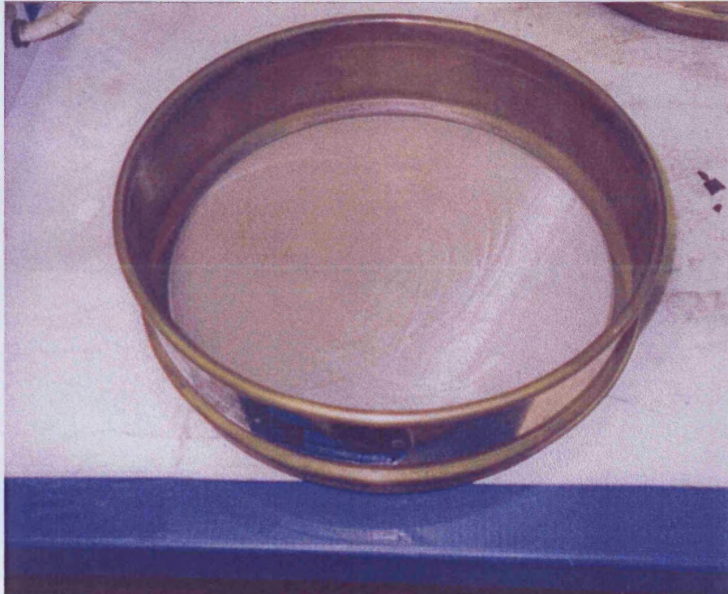
Sieve used in size distribution process
