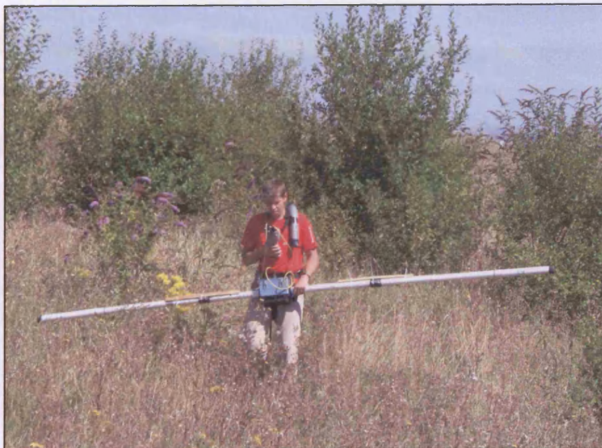
Figure 2.12: A photograph illustrating the Geonics EM31, utilised for environmental investigations requiring depths of around ~5 metres (photograph by Dr. P. Brabham, Cardiff University).
