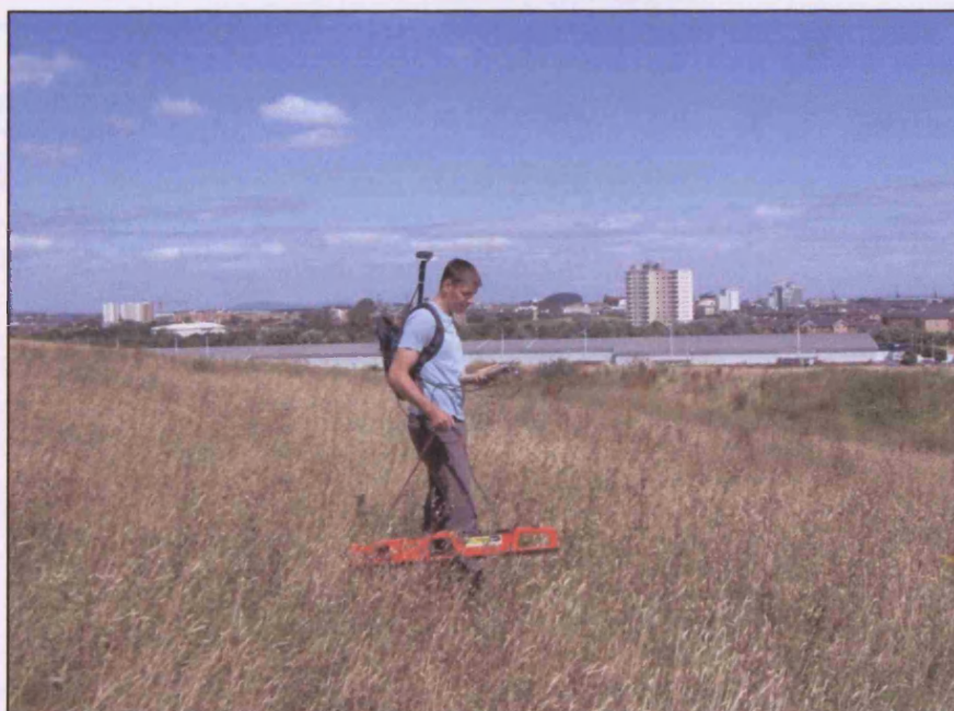
Figure 2.13: A photograph illustrating the Geonics EM38, utilised for shallow environmental investigations to around ~1 metre depth (photograph by Dr. P. Brabham, Cardiff University).
