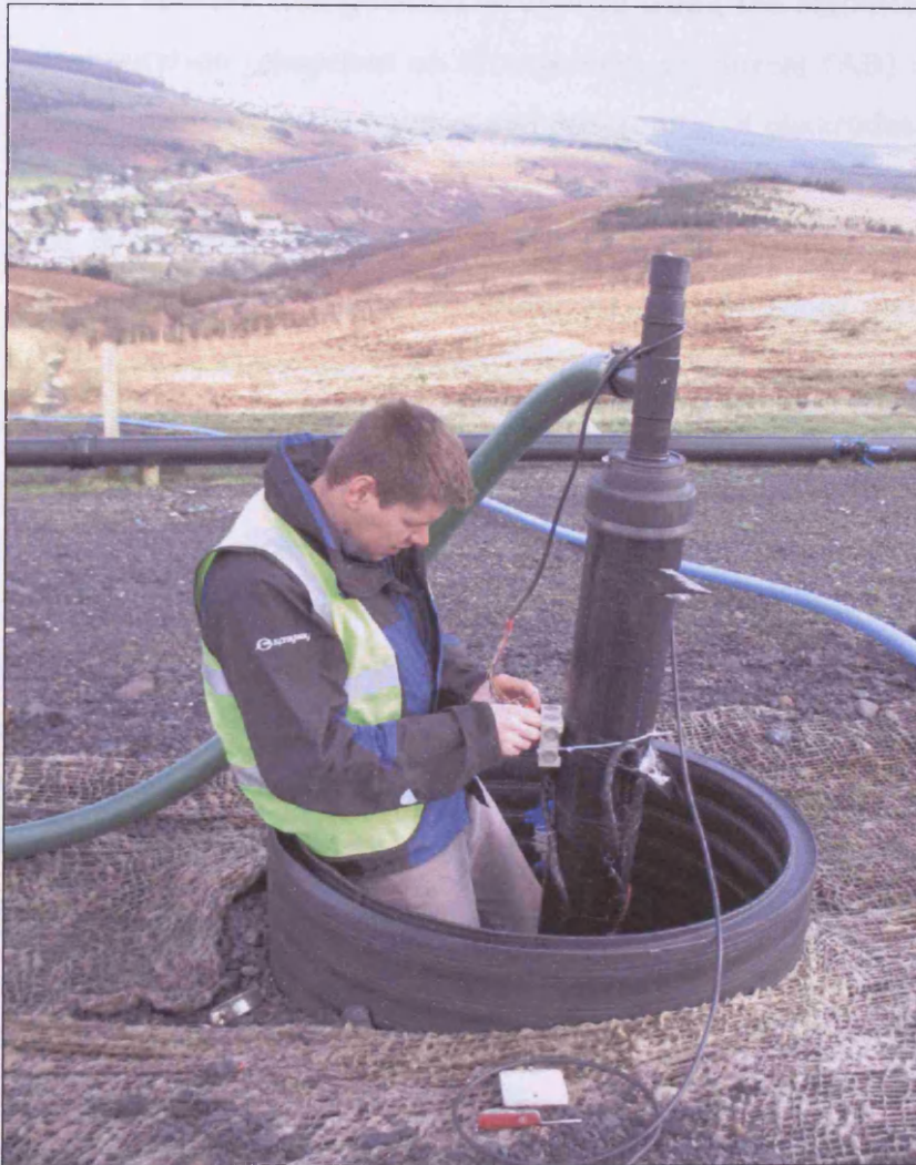
Figure 6.6: A photograph illustrating the electrode array connection box mounted at each gas well head for connection to the ERT instrument (Dr. P. Brabham, Cardiff University).
