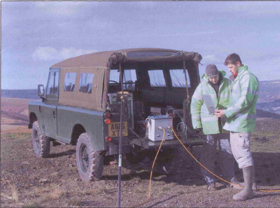
Figure 3.26: A photograph illustrating the ERT measurement equipment in use during the reconnaissance survey in February 2004 (author).
