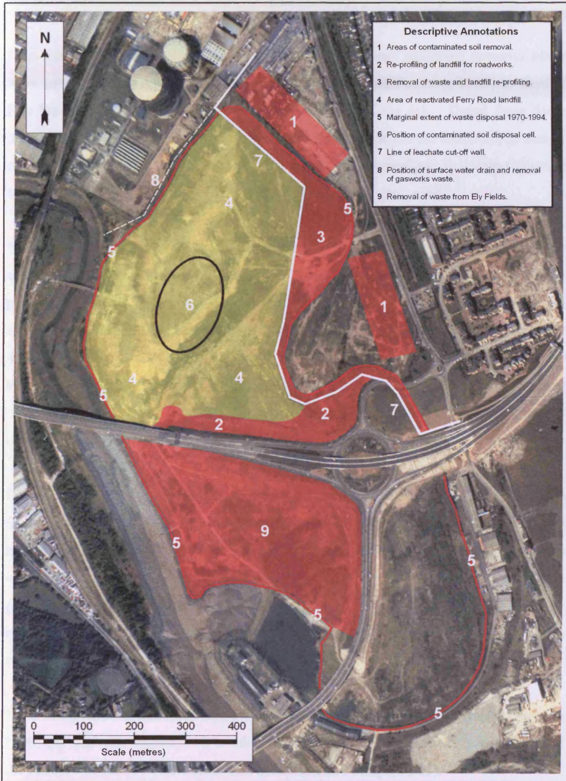
Figure 3.7: An illustrated air photograph of the Ferry Road landfill and adjoining areas showing detail of the site reactivation between 1996 to 1999.
