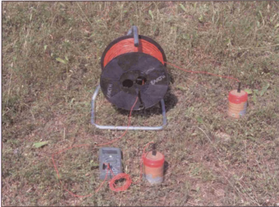
Figure 2.9: A photograph illustrating the non-polarising electrodes and voltmeter used during Self-Potential surveys (author).
