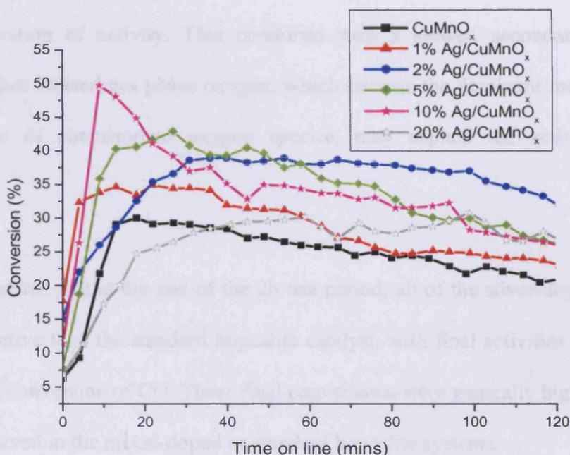
Figure 4.2.3.1 – CO oxidation activity of silver-doped  $\text{CuMnO}_x$  catalysts aged for 30 minutes as a function of percentage silver doping
