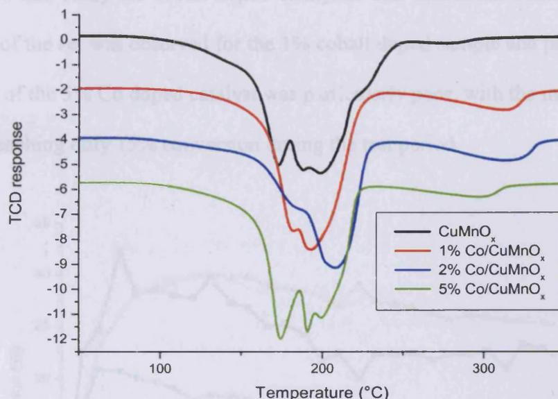
Figure 5.3.1 – TPR profiles of 1h aged Co doped CuMnO<sub>x</sub> catalysts
