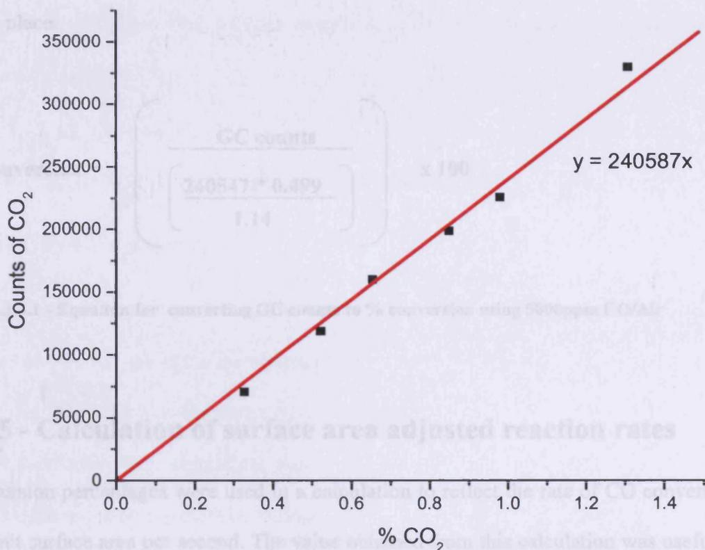
Figure 2.2.3.1 – Calibration of GC using mixtures of known CO<sub>2</sub> concentration
