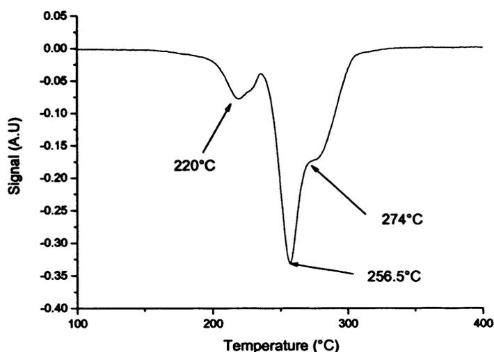
**Figure 3. 1.4.1 - A TPR trace of CuMnO<sub>x</sub>, calcined at 500°C, 17h carried out in 10% H<sub>2</sub>/Ar with a 10°C/min ramp rate**
