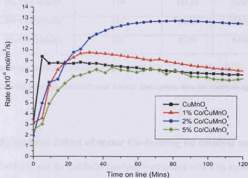
Figure 5.6.4.2 – Surface area adjusted reaction rates for CO oxidation over 6h aged Co doped CuMnO<sub>x</sub> catalysts
