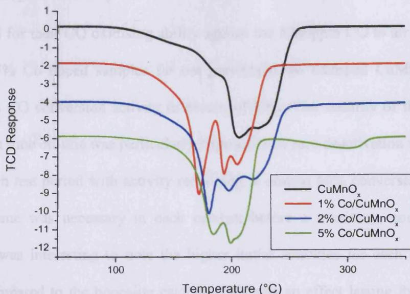
**Figure 5.1.2.1 – TPR profiles of Co doped  $\text{CuMnO}_x$  catalysts**
