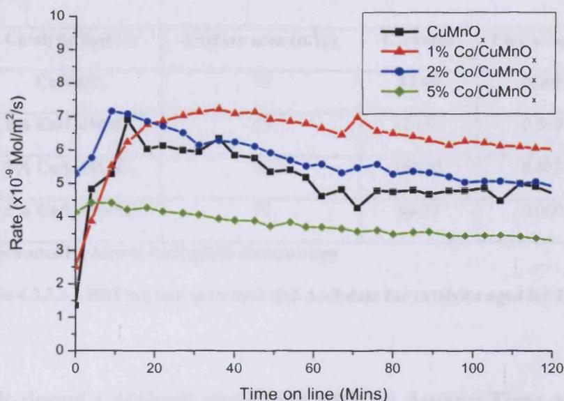
**Figure 5.3.3 – Surface area adjusted reaction rates for CO oxidation over 1h aged Co doped CuMnO<sub>x</sub> catalysts**
