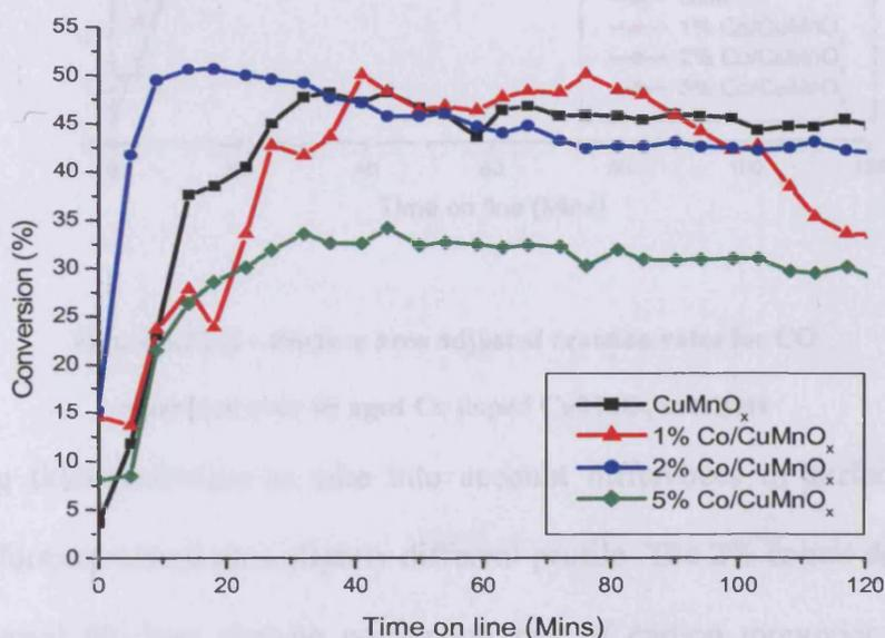
Figure 5.5.3.1 – CO oxidation activity of 4h aged Co doped CuMnO<sub>x</sub> catalysts
