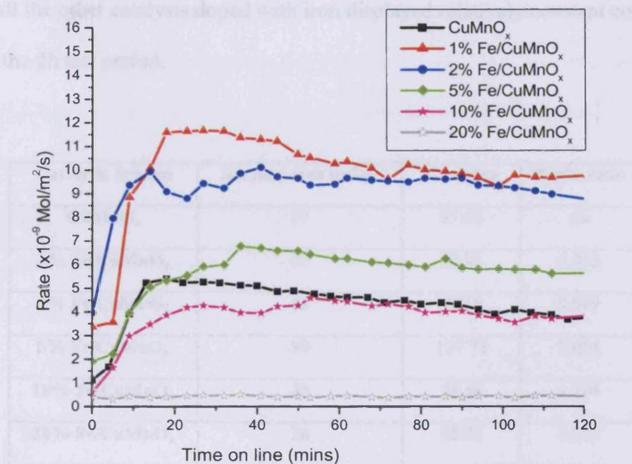
Figure 4.4.2.2 – Surface area adjusted reaction rates for CO oxidation over Fe doped CuMnO<sub>x</sub> catalysts aged for 30 minutes
