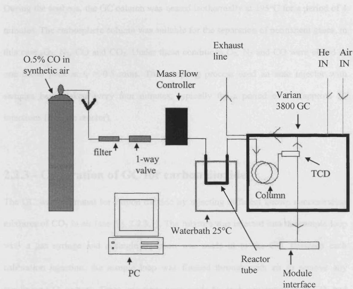
Fig 2.2.2.1 – Schematic of the micro reactor system for the CO/Air test mixture
