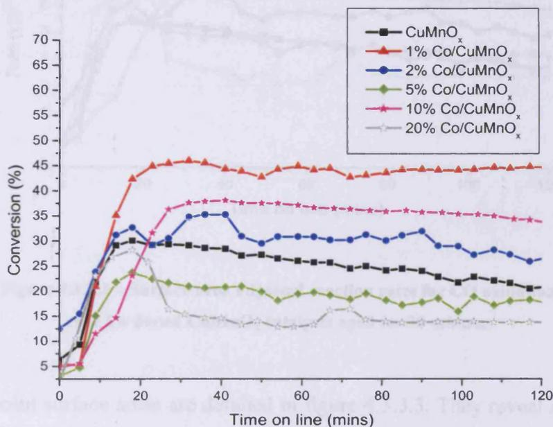
Figure 4.3.3.1 – CO oxidation activity a series of Co doped CuMnO<sub>x</sub> catalysts aged for 30 minutes
