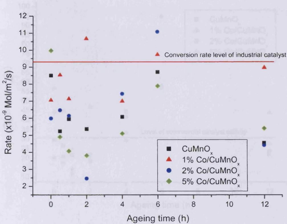
Figure 5.8.1.4 – surface area adjusted rate of CO conversion after 30 minutes on-line as a function of ageing time and % cobalt doping
