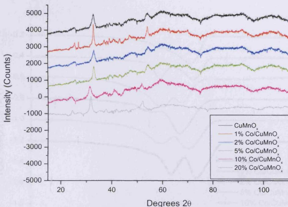
Figure 4.3.1.1 – X-ray diffraction data of cobalt-doped  $\text{CuMnO}_x$ , as a function of % Co doping
