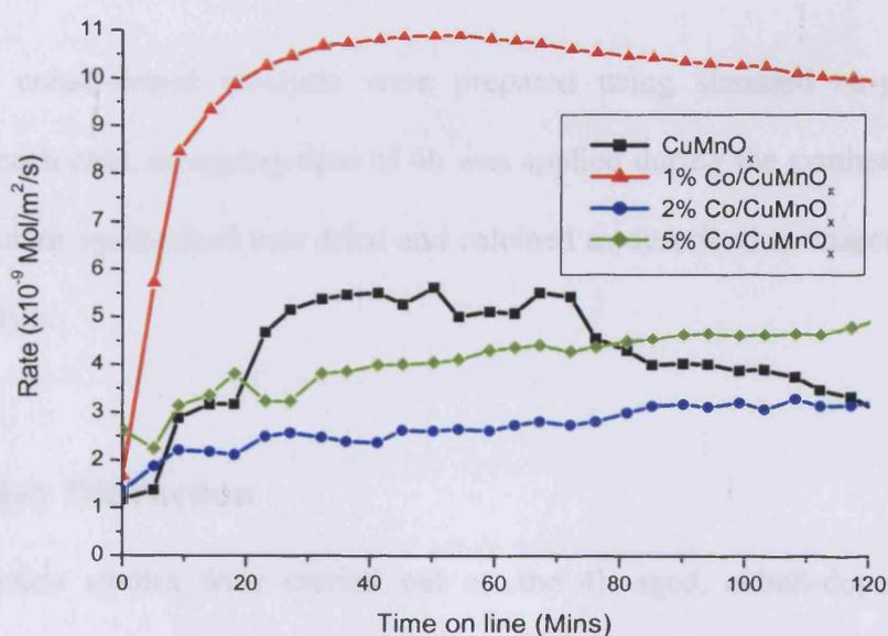
Figure 5.4.3.2 – Surface area adjusted reaction rates for CO oxidation over 2h aged Co doped CuMnO<sub>x</sub> catalysts
