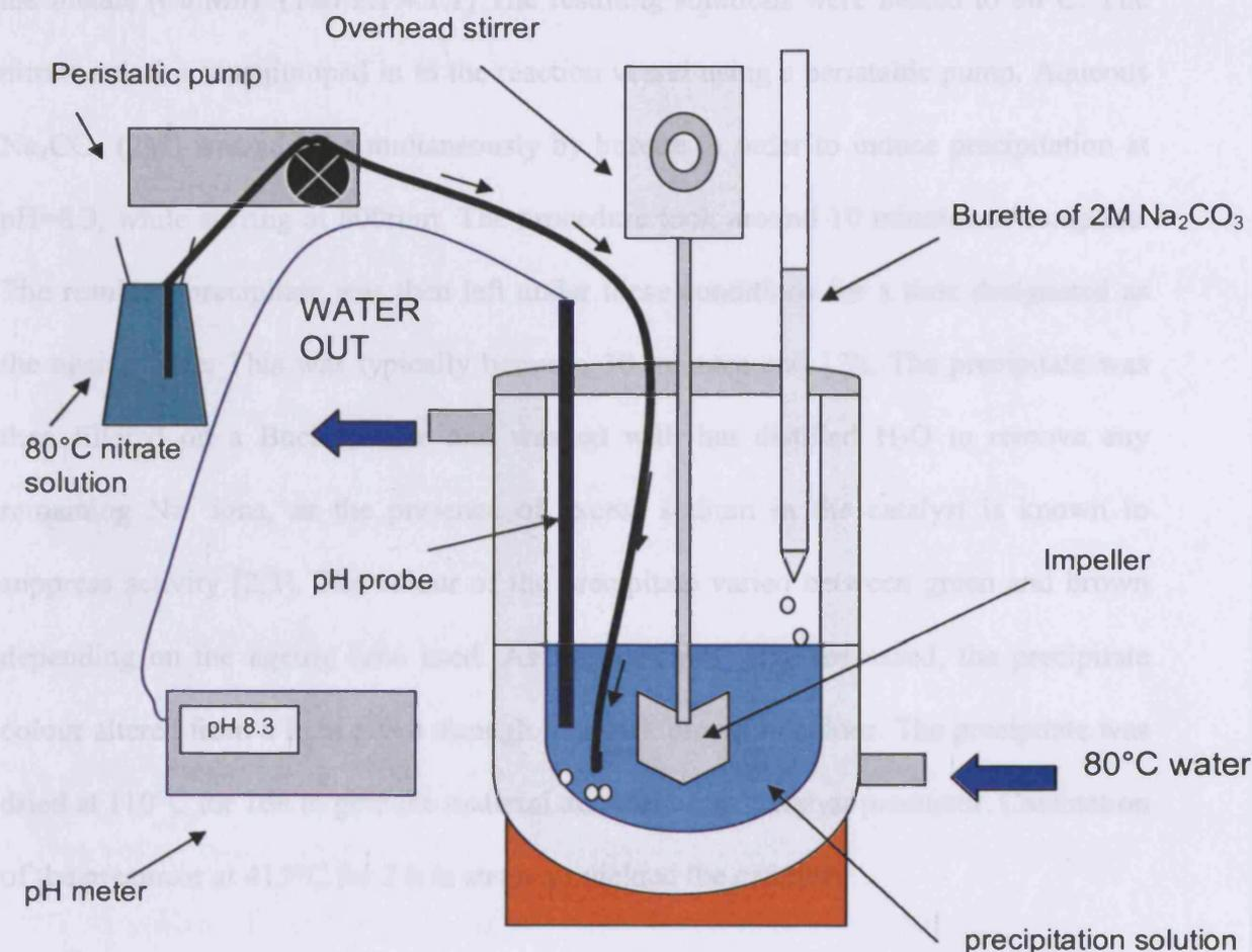
Figure 2.1.2.1 – Diagram of modified co-precipitation apparatus
