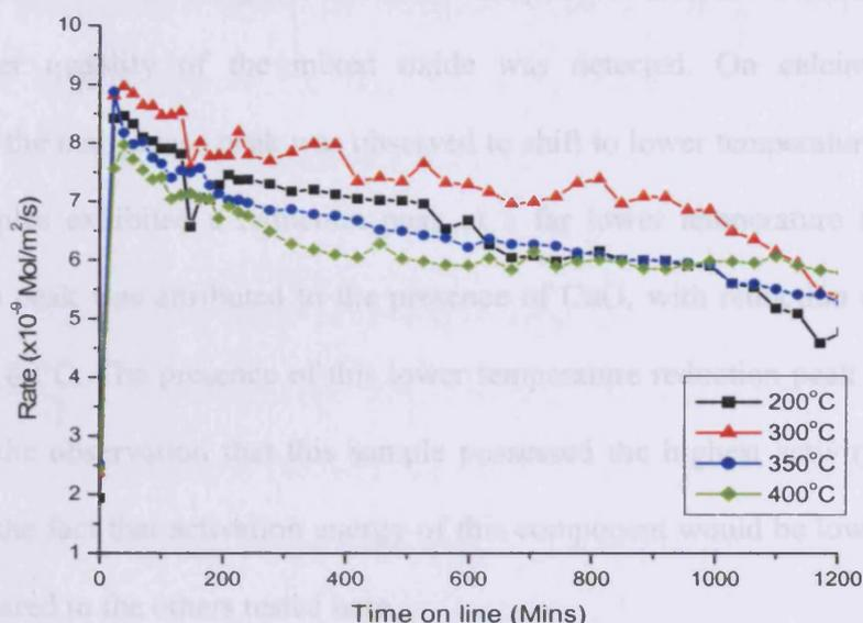
Figure 3.2.4.2 – Surface area adjusted reaction rates for CO oxidation at 25°C as a function of calcination temperature
