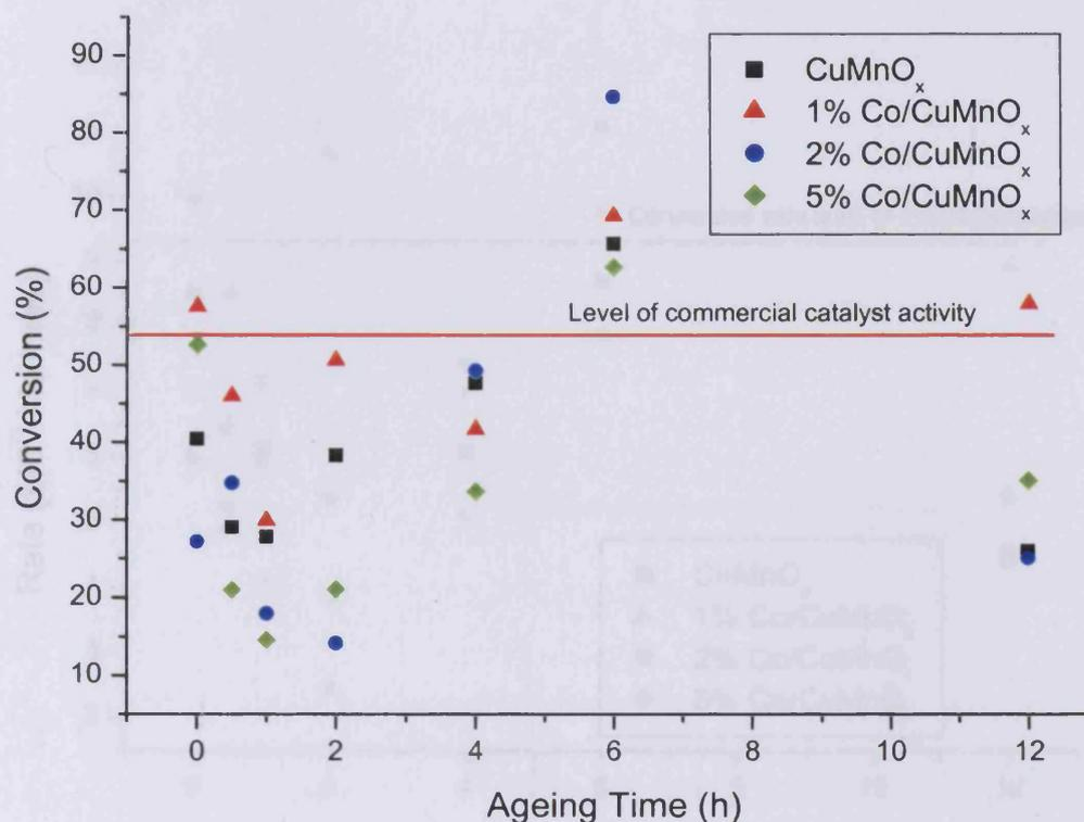
Figure 5.8.1.3 – Comparison of start-up activity levels after 30 minutes on-line as a function of ageing time and % cobalt doping
