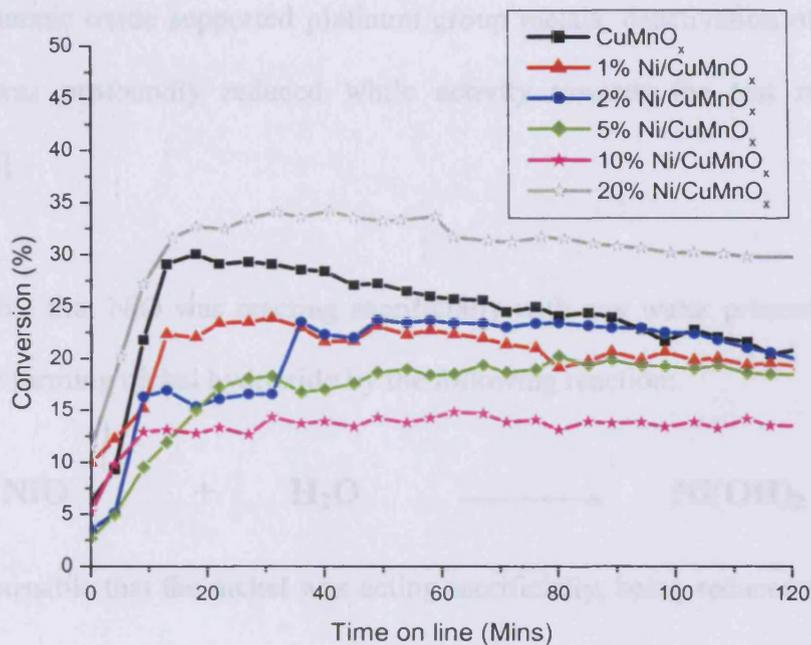
Figure 4.1.3.1 – CO oxidation activity a series of Ni doped  $\text{CuMnO}_x$  catalysts aged for 30 minutes
