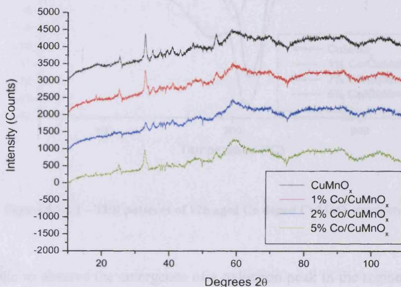
Figure 5.7.1.1 – XRD of 12h aged Co doped CuMnO<sub>x</sub> catalyst precursors dried at 100°C, 16h
