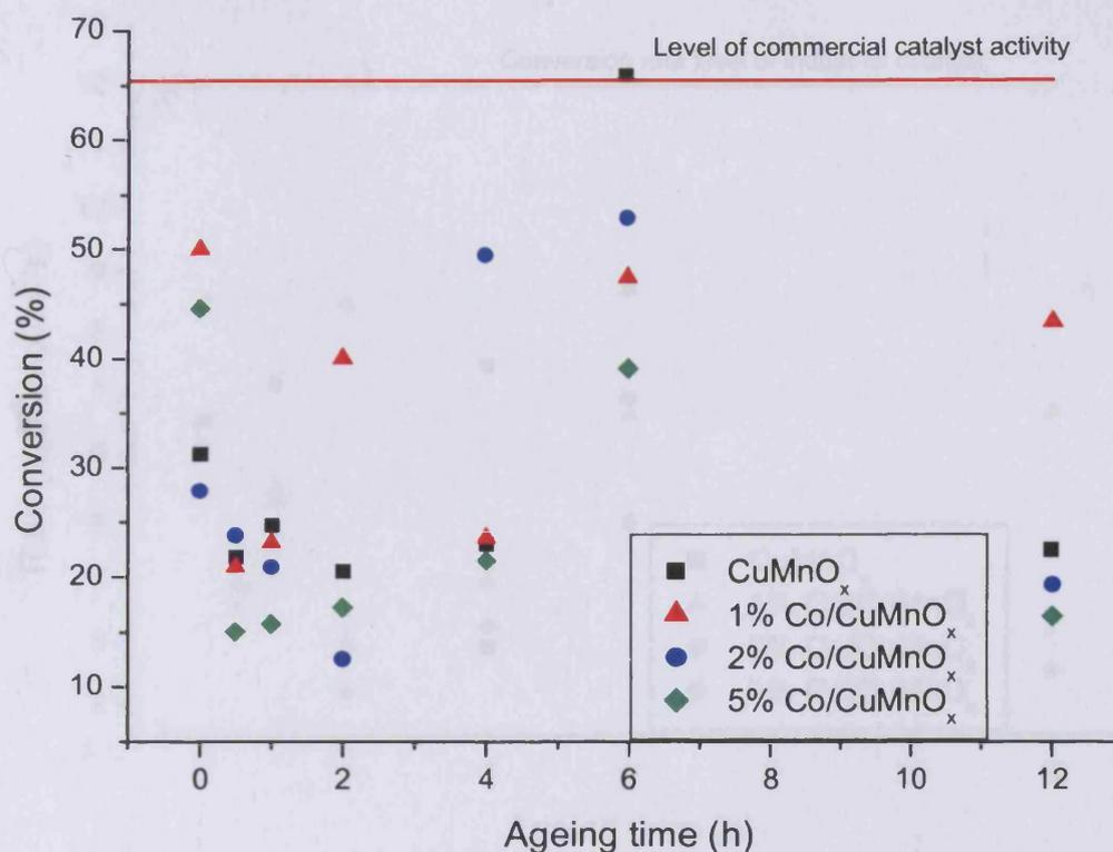
Figure 5.8.1.1– Comparison of start up activity levels after 10 minutes on-line as a function of ageing time and % cobalt doping
