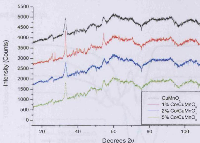
Figure 5.2.1.1 – X-ray diffraction patterns of Co doped CuMnO<sub>x</sub> as a function of % Co doping
