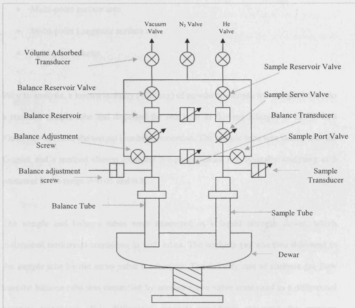
Figure 2.3.3.3 – Schematic of Gemini 2360 analyser
