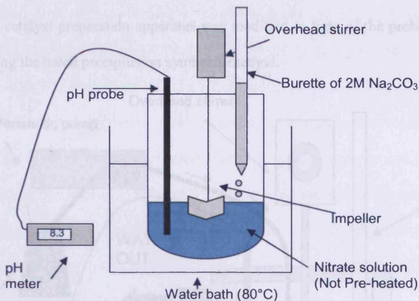
Figure 2.1.1.1 – Diagram of original co-precipitation apparatus
