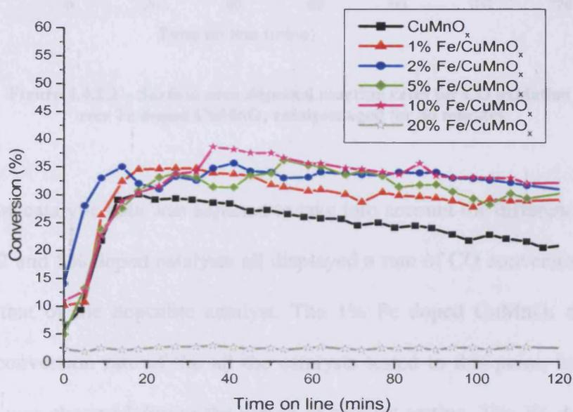
Figure 4.4.2.1 – CO oxidation activity of iron-doped  $\text{CuMnO}_x$  catalysts aged for 30 minutes
