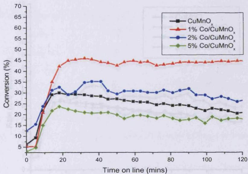
Figure 5.2.3.1 – CO oxidation activity of 0.5h aged Co doped CuMnO<sub>x</sub> catalysts
