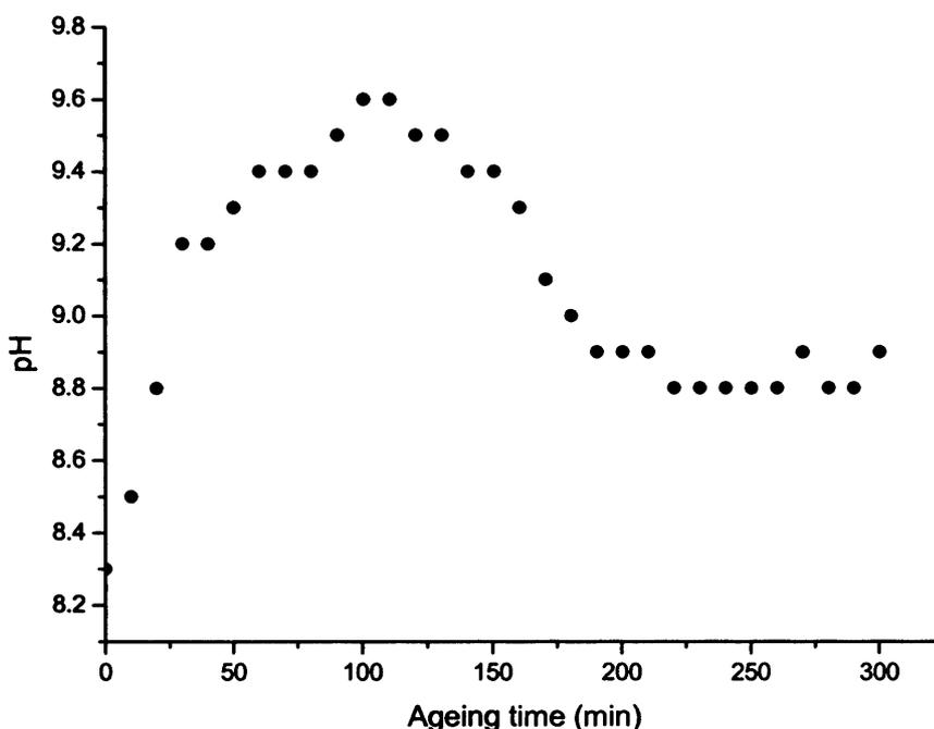
Figure 3.5.1.1- pH drift profile during the precipitate ageing process
