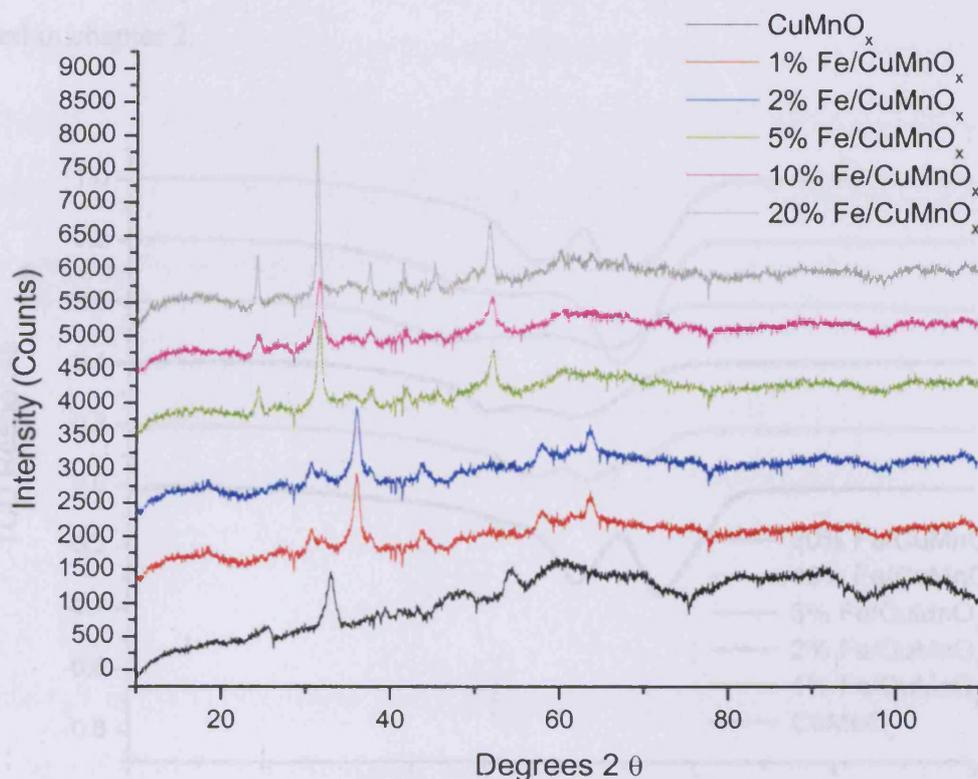
Figure 4.4.1.1 – X ray diffraction patterns of Fe doped CuMnO<sub>x</sub>
