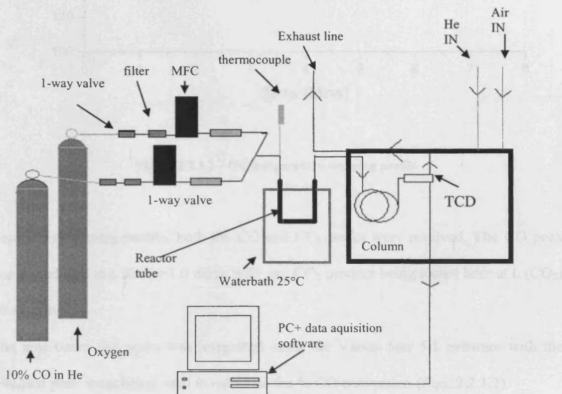
Figure 2.2.1.1 - Schematic of the microreactor system
