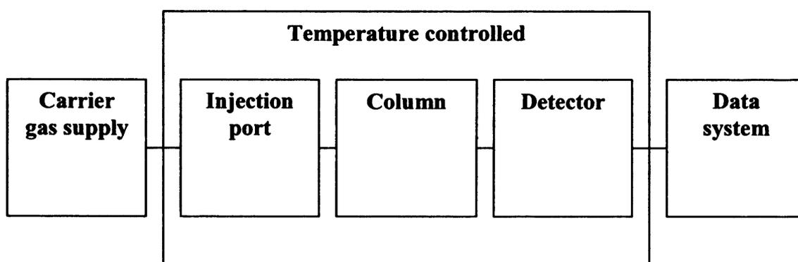
Figure 2.3.1.1 – Block diagram of a gas chromatograph
