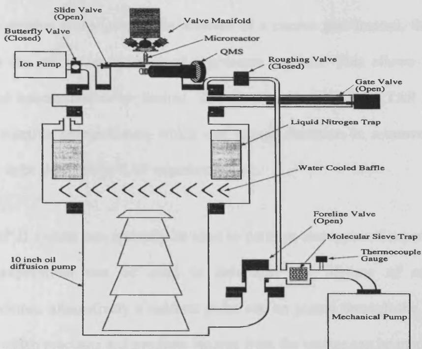
Figure 6.1.1 – Schematic diagram of a TAP II
