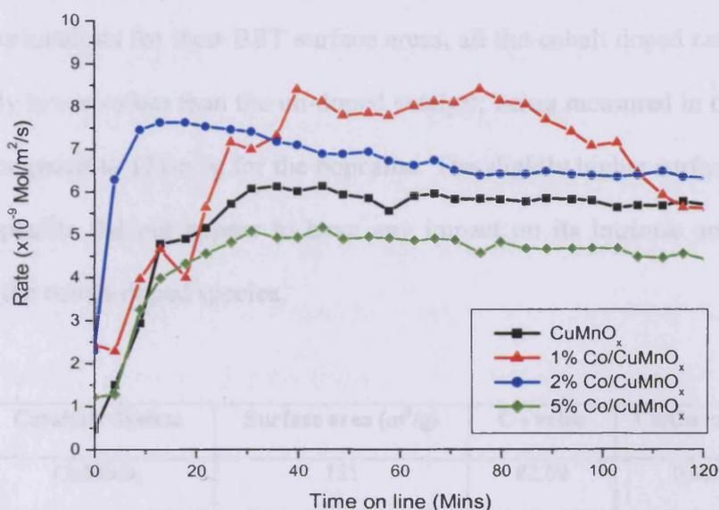
**Figure 5.5.3.2 – Surface area adjusted reaction rates for CO oxidation over 4h aged Co doped CuMnO<sub>x</sub> catalysts**
