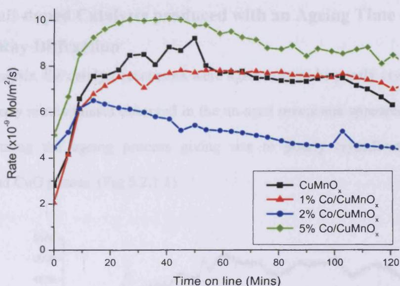
Figure 5.1.3.2 – Surface area adjusted reaction rates for CO oxidation over Co doped  $\text{CuMnO}_x$  catalysts aged for 0h
