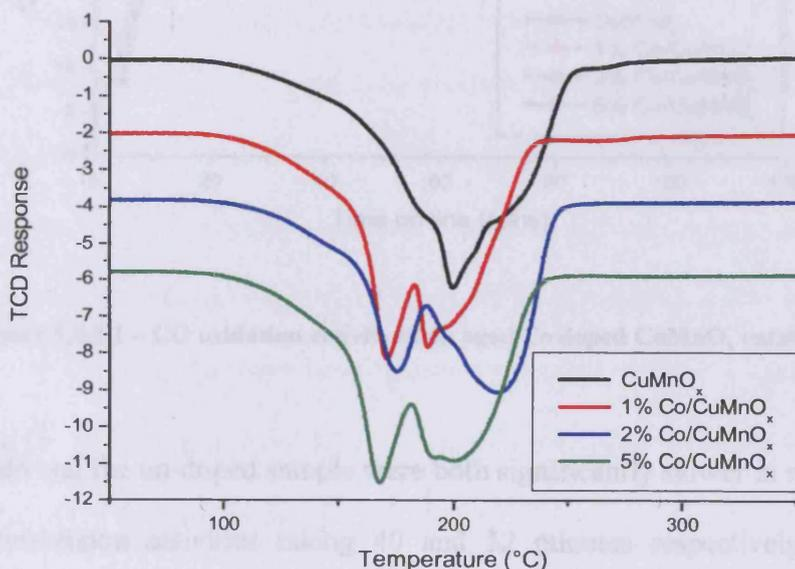
Figure 5.5.2.1 – TPR patterns of 4h aged Co doped CuMnO<sub>x</sub> catalysts
