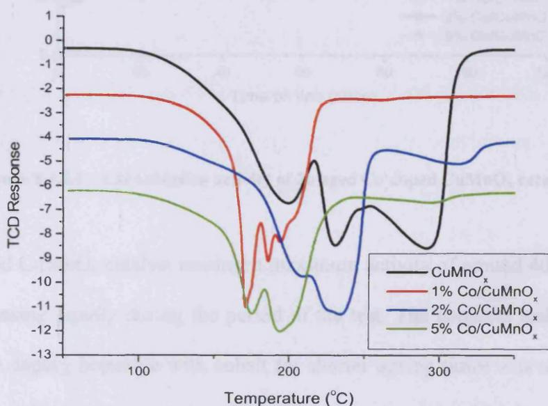
Figure 5.4.2.1 - TPR patterns of 2h aged Co doped CuMnO<sub>x</sub> catalysts
