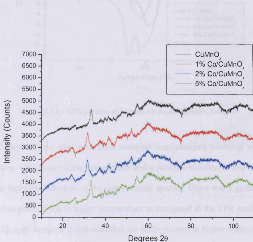
Figure 5.3.1.1 – XRD pattern of 1h aged Co doped CuMnO<sub>x</sub> catalysts
