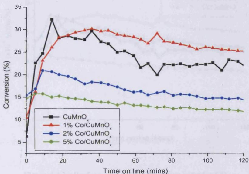
Figure 5.3.3.1 – CO oxidation activity of 1h aged Co doped CuMnO<sub>x</sub> catalysts
