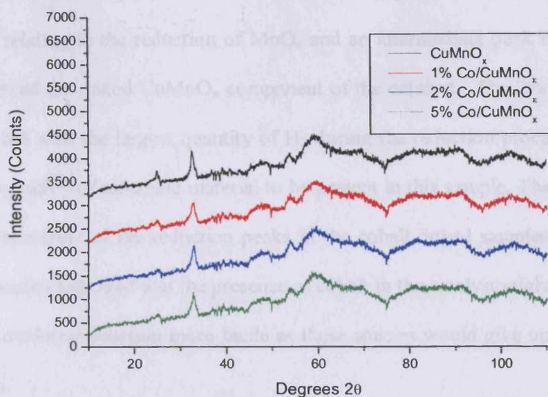
**Figure 5.5.1.1 – XRD pattern of 4h aged Co doped CuMnO<sub>x</sub> catalyst precursors dried at 100°C, 16h**
