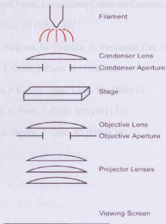
**Figure 2.3.7.1 – Schematic of an electron microscope**
