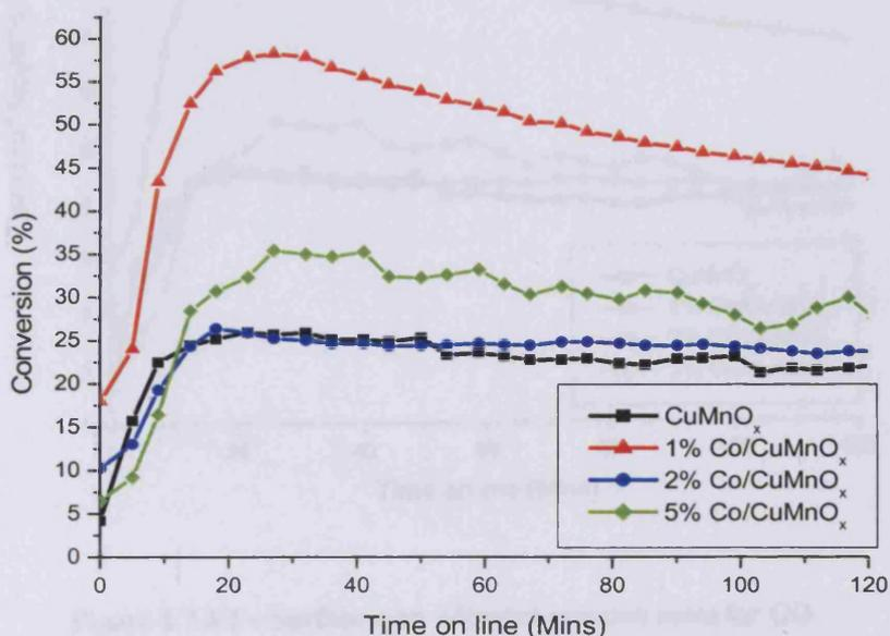
Figure 5.7.3.1 – CO oxidation activity of 12h aged Co doped CuMnO<sub>x</sub> catalysts
