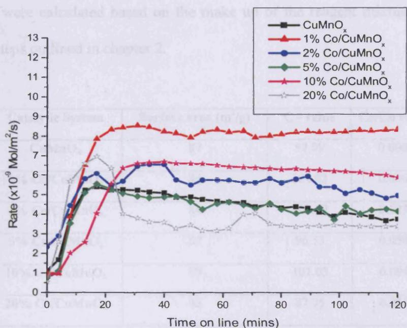
Figure 4.3.3.2 – Surface area adjusted reaction rates for CO oxidation over Co doped CuMnO<sub>x</sub> catalysts aged for 30 minutes
