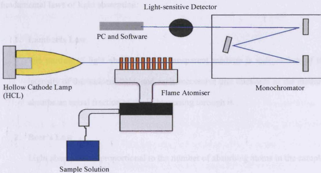
Figure 2.3.6.1 – Schematic of a typical Atomic Absorption Spectrometer
