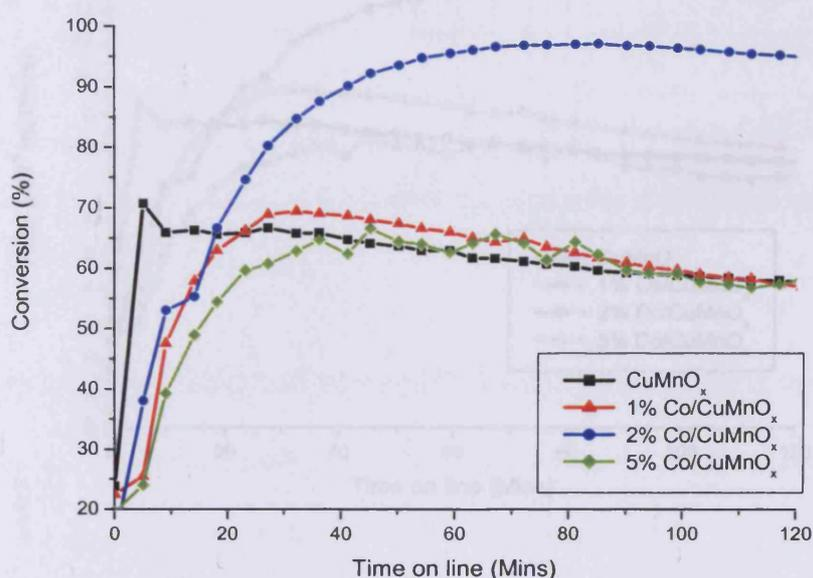
Figure 5.6.4.1 – CO oxidation activity of 6h aged Co doped CuMnO<sub>x</sub> catalysts
