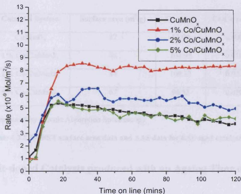
Figure 5.2.3.2 – Surface area adjusted reaction rates for CO oxidation over 0.5h aged Co doped CuMnO<sub>x</sub> catalysts
