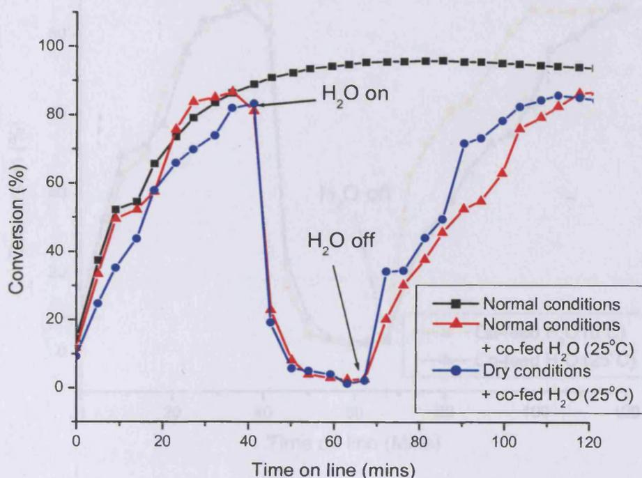
Figure 5.6.5.1.1 – Water co-feeding experiments over 2% cobalt doped CuMnO<sub>x</sub>, 6h aged
