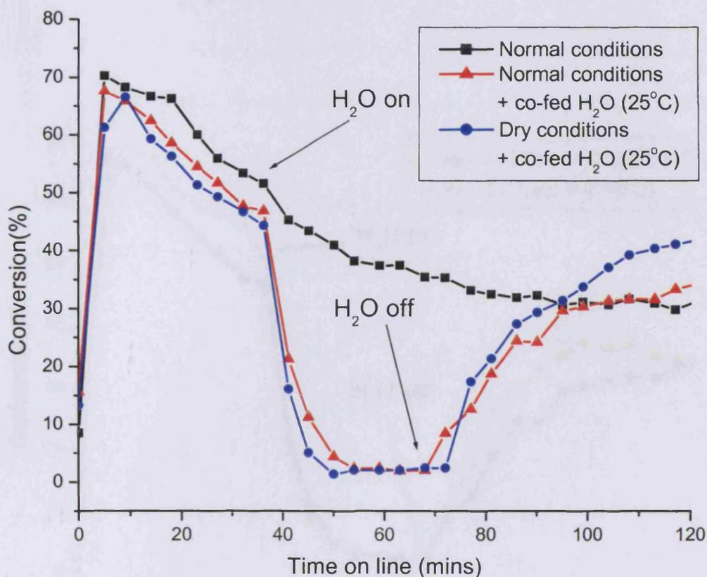
Figure 5.6.5.2.1 - Water co-feeding experiments over Moleculte
