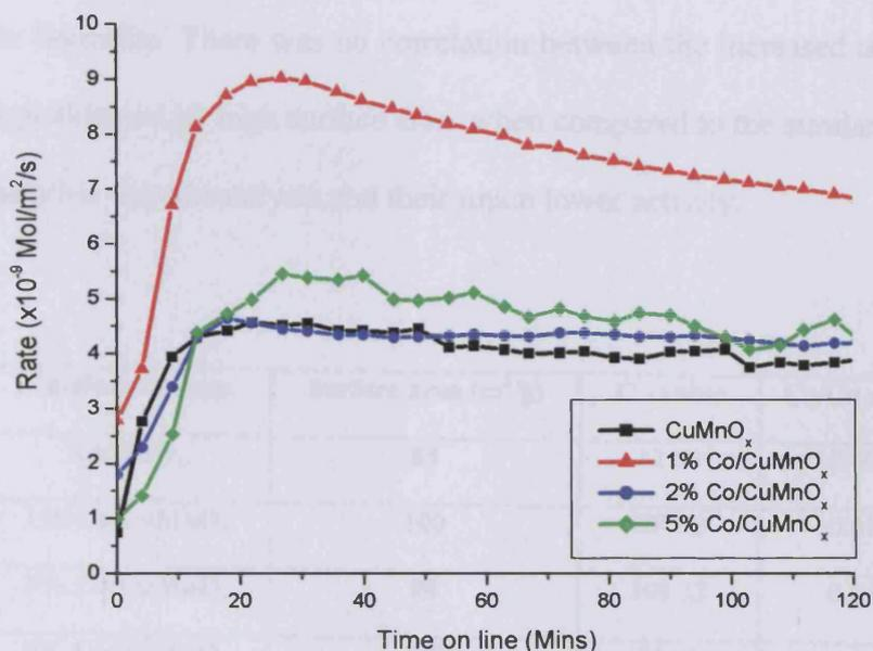
**Figure 5.7.3.2 – Surface area adjusted reaction rates for CO oxidation over 12h aged Co doped CuMnO<sub>x</sub> catalysts**
