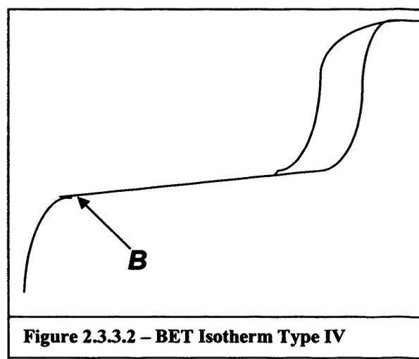
The experiment is carried out by measuring the amount of  $N_2$  adsorbed on the sample at 77K as a function of the pressure of the  $N_2$  over the sample. The final surface area is determined by assuming that each molecule of adsorbed nitrogen occupies an area of  $0.165nm^2$ . BET plots are normally carried out in the range  $(P/P_0)= 0.05$  to  $0.35$  with 1, 3 or most commonly 5 points in the isotherm range.
