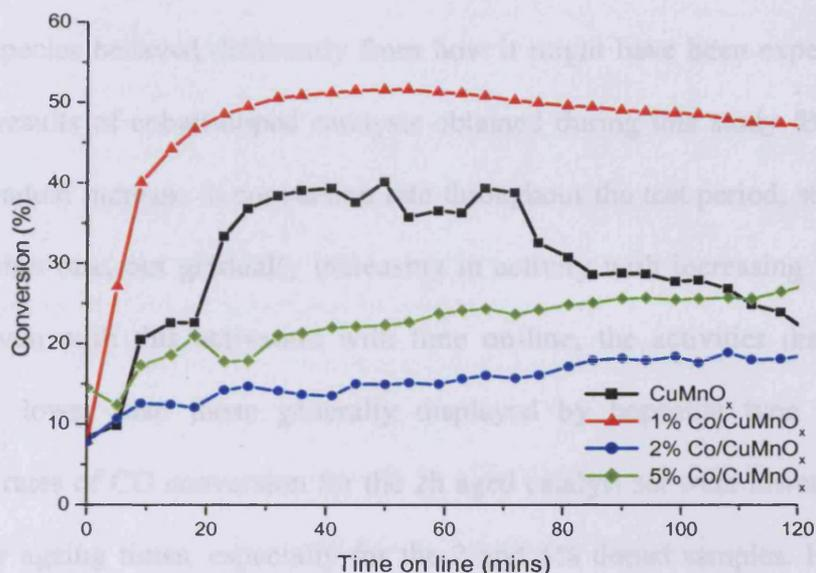
Figure 5.4.3.1 – CO oxidation activity of 2h aged Co doped CuMnO<sub>x</sub> catalysts
