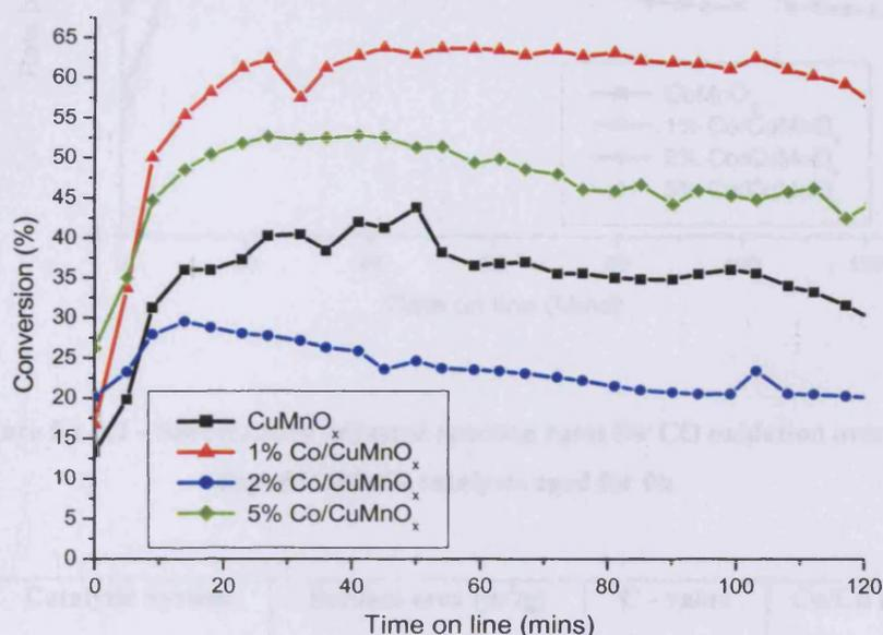
Figure 5.1.3.1 – CO oxidation activity a series of Co doped  $\text{CuMnO}_x$  catalysts aged for 0h
