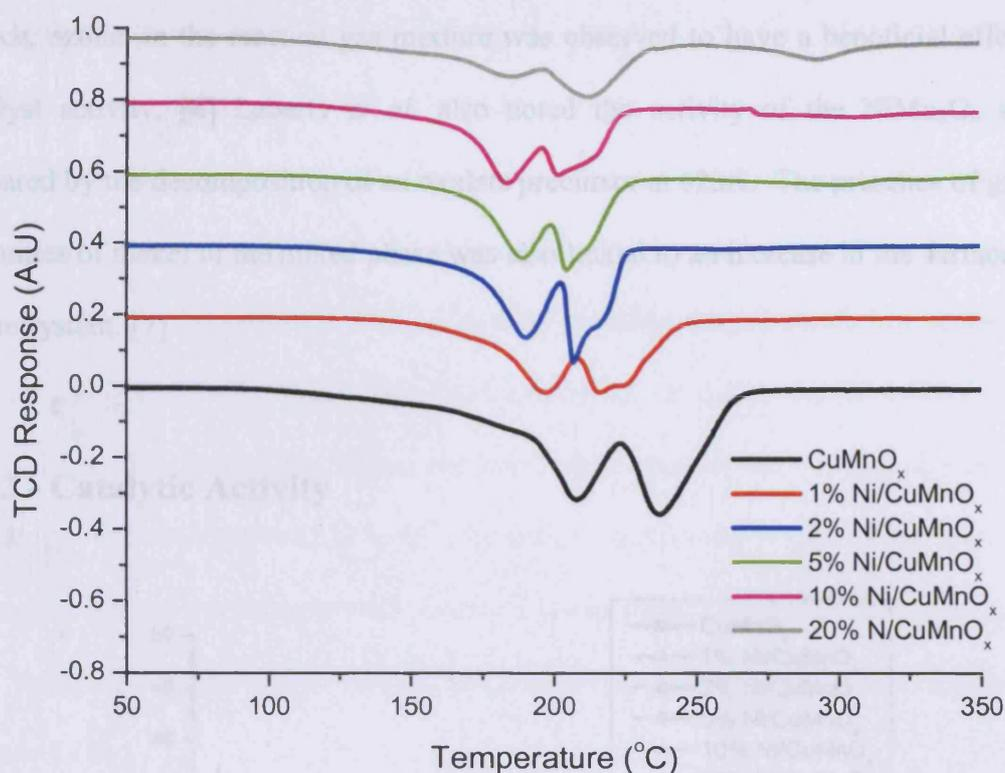
Figure 4.1.2.1 - TPR profiles of nickel-doped  $\text{CuMnO}_x$  catalysts calcined at  $415^\circ\text{C}$  for 2h as a function of % cobalt doping
