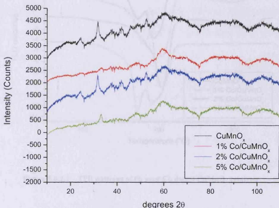
Figure 5.6.1.1 – XRD patterns of 6h aged Co doped CuMnO<sub>x</sub>
