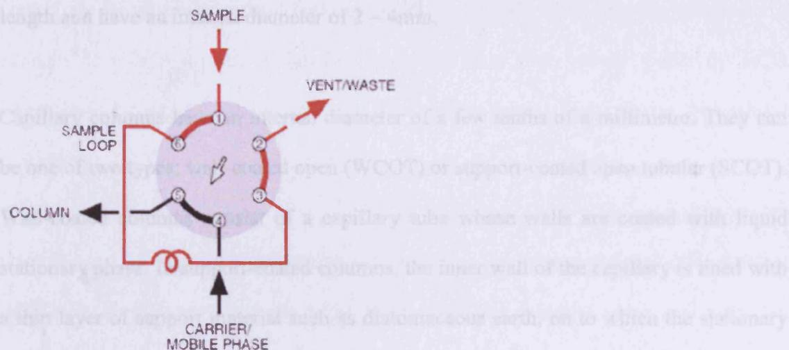
**Figure 2.3.1.2.1- Position A: Auto injector “FILL” mode**
