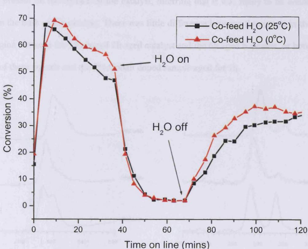
Figure 5.6.5.2.2 - Water co-feeding experiments over Moleculte
