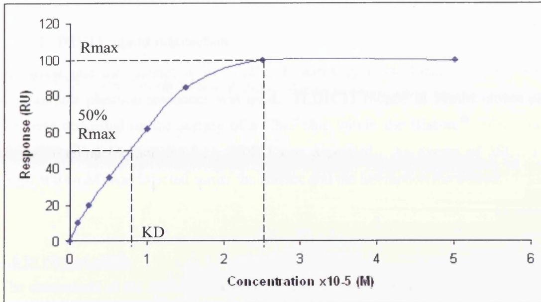
**Figure 2.5 Calculation of Rmax and KD**
