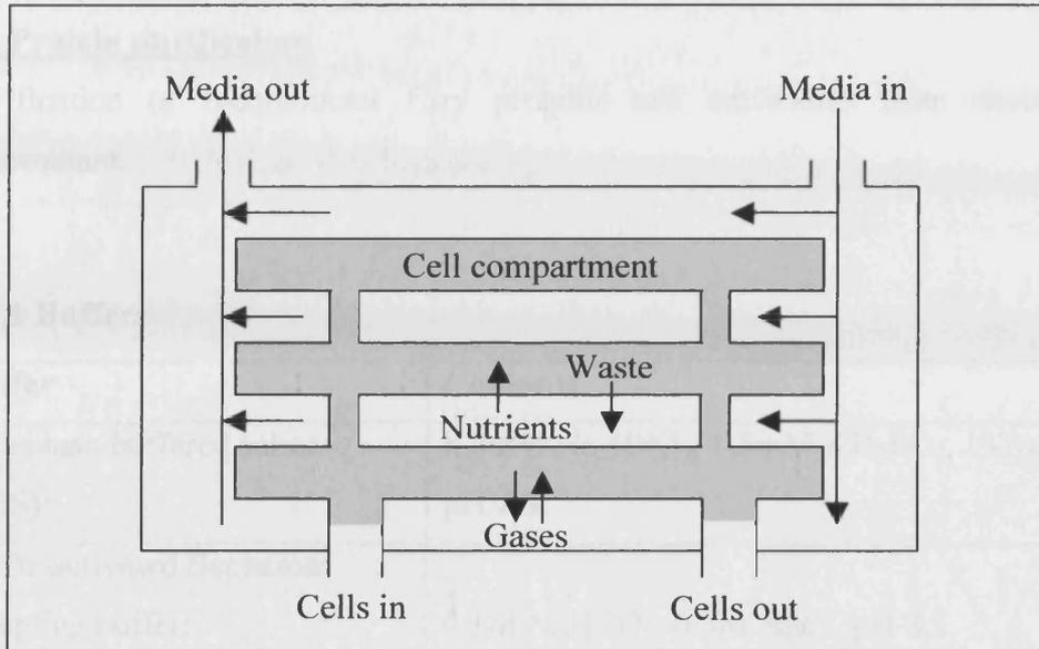
**Figure 2.3 Diagram of the Tecnomouse cassette.**
