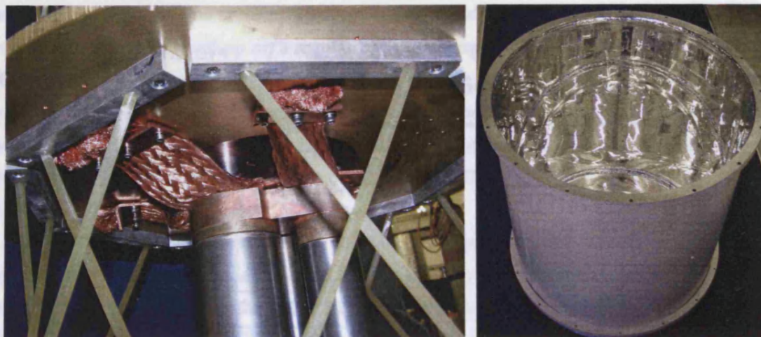
Figure 2.3: The left picture shows how the thermal straps connect the PTC cold head to the base plate. The right picture shows the vacuum can with its internal surface covered with sheets of aluminized mylar.
