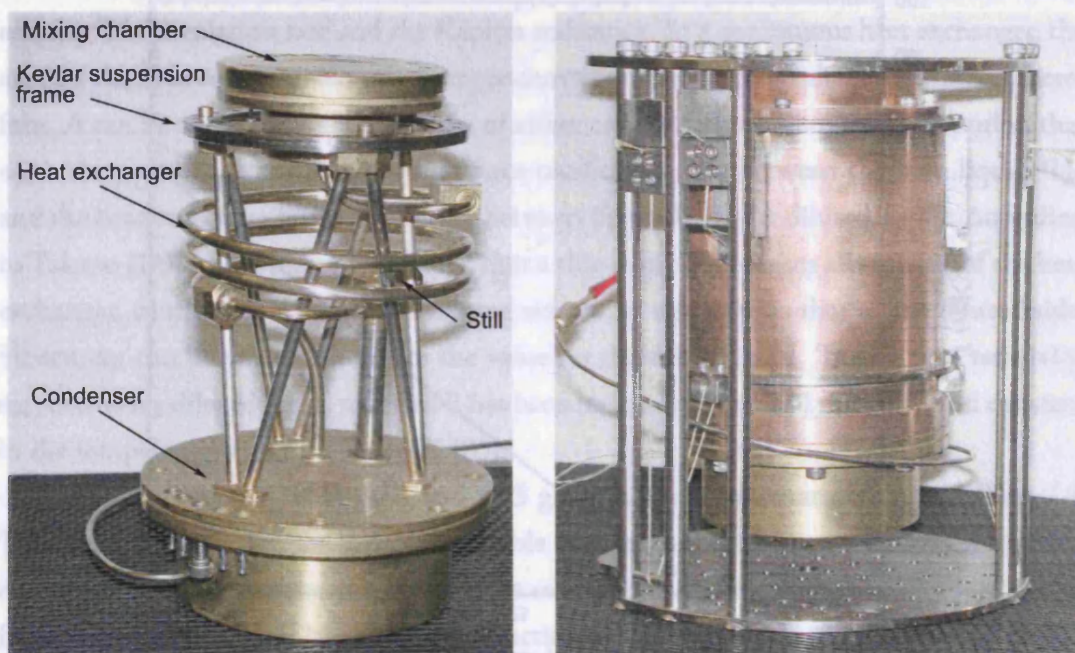
Figure 4.6: Two pictures of the MDR developed during this project. The left picture shows the principle components of the MDR, and the right picture shows the MDR with its radiation shield suspended with Kevlar
