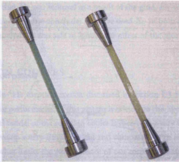
Figure 2.10: A picture of the G10 (green) and Epoxy (yellow) rod samples used for the tension test. The compression test samples were plain rods without any end caps.
