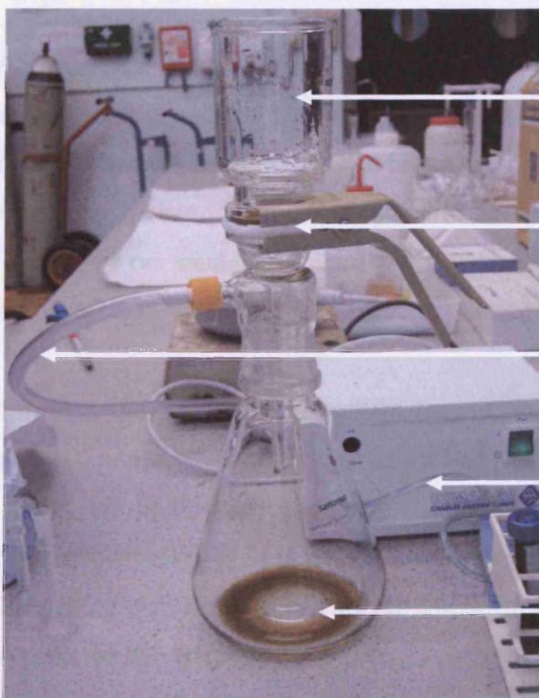
Figure 7.2: Filtering Step; Sartorius filter unit and pump.
