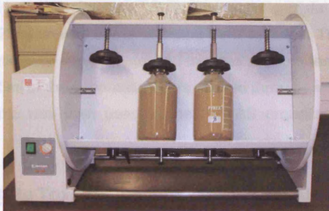
Figure 7.1: Leaching step; end-over-end tumbler.
