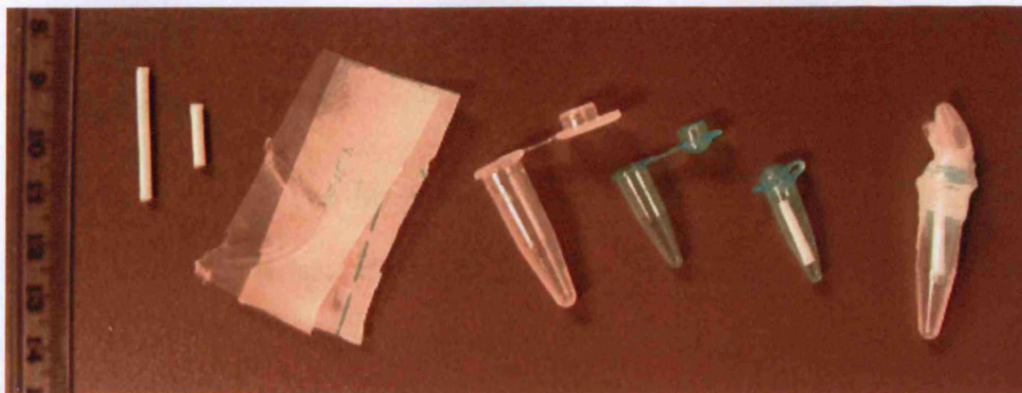
Figure 2.1 Preparing polyester rod material samples for centrifugation
