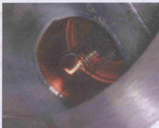
Fig. 2.6: An ion gauge retracted under working conditions inside a UHV chamber.
