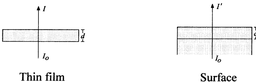
Fig. 2.18: The detected photoelectron flux passing through a thin film (thickness d ), and originating from within a surface depth ( d ).
