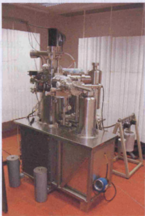
Figure 2-28 – Super-STEM system at Daresbury.
