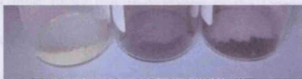
Figure 4-18 - Mo:Fe 2.2:1 catalyst pre reduction, after reduction with 60 µl methanol at 250 °C and 330 °C.
