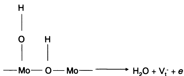
Figure 3-24 - Suggested mechanism for the formation of H 2 O on the surface of MoO 3 20 .
