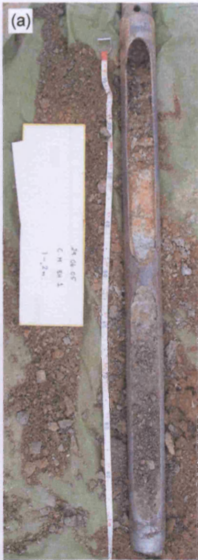
Figure 6.8: Photographs of sediments from Borehole 1 and Borehole 2, Crychell Moor: (a) Sandy fine gravel (diamict), with gravelly silty sand (1.3-1.65 m), 1-2 m, Borehole 1; (b) Silty sandy gravel (diamict), 3-4 m, Borehole 1; (c) Clayey silt, 3-4 m, Borehole 2.
