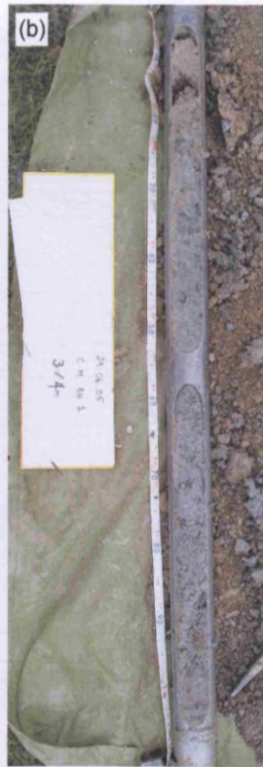
Figure 6.8: Photographs of sediments from Borehole 1 and Borehole 2, Crychell Moor: (a) Sandy fine gravel (diamict), with gravelly silty sand (1.3-1.65 m), 1-2 m, Borehole 1; (b) Silty sandy gravel (diamict), 3-4 m, Borehole 1; (c) Clayey silt, 3-4 m, Borehole 2.
