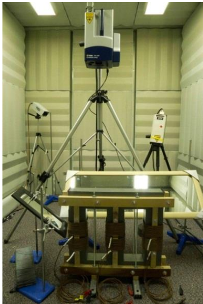
Fig.4-17: Photograph of the vibration measurement system
