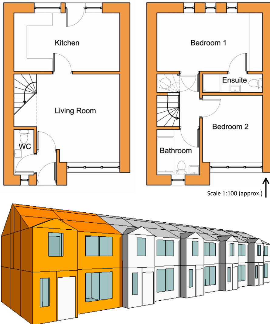
Figure 26 Floor plans and IES model view showing end terrace dwelling (South elevation)
