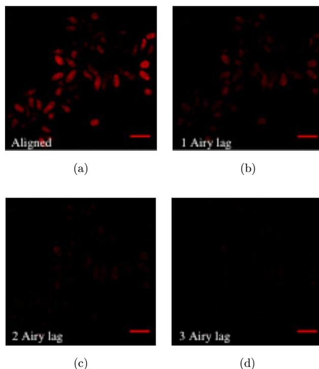
Fig. 7. Two-photon laser scanning confocal images of Ru nanoparticle-electroporated *S. pombe* acquired by using (a) the optically-aligned excitation beam, (b)–(d) the pinhole shift giving displacement by 1, 2 or 3 Airy units, respectively. Scale bars =  $10 \mu\text{m}$  Reproduced with permission from Williams *et al.*<sup>48</sup>
