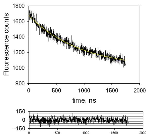
Fig. 8. Typical phosphorescence trace of Ru complex-loaded nanoparticles taken up by HDF cells. The value of the lifetime was  $0.93 \mu\text{s}$ . The fitted line is shown as the smooth line. The bottom panel shows the residuals: these were due to the background counts recorded in complete darkness. Reproduced with permission from Williams *et al.*<sup>48</sup>
