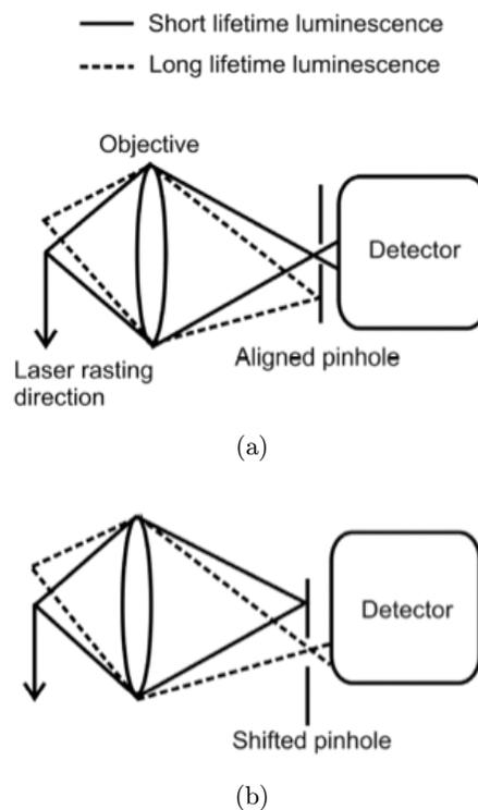
Fig. 1. The pinhole shifting technique. By shifting the pinhole successively out of its optimally aligned position (a), through a series of steps (e.g., b), collection of sequential time-delayed phosphorescence emission in the lagging direction of the raster scanned two-photon excitation is achieved by employing appropriate laser beam scanning speeds. Reproduced with permission from Ramshesh 2007.<sup>50</sup>
