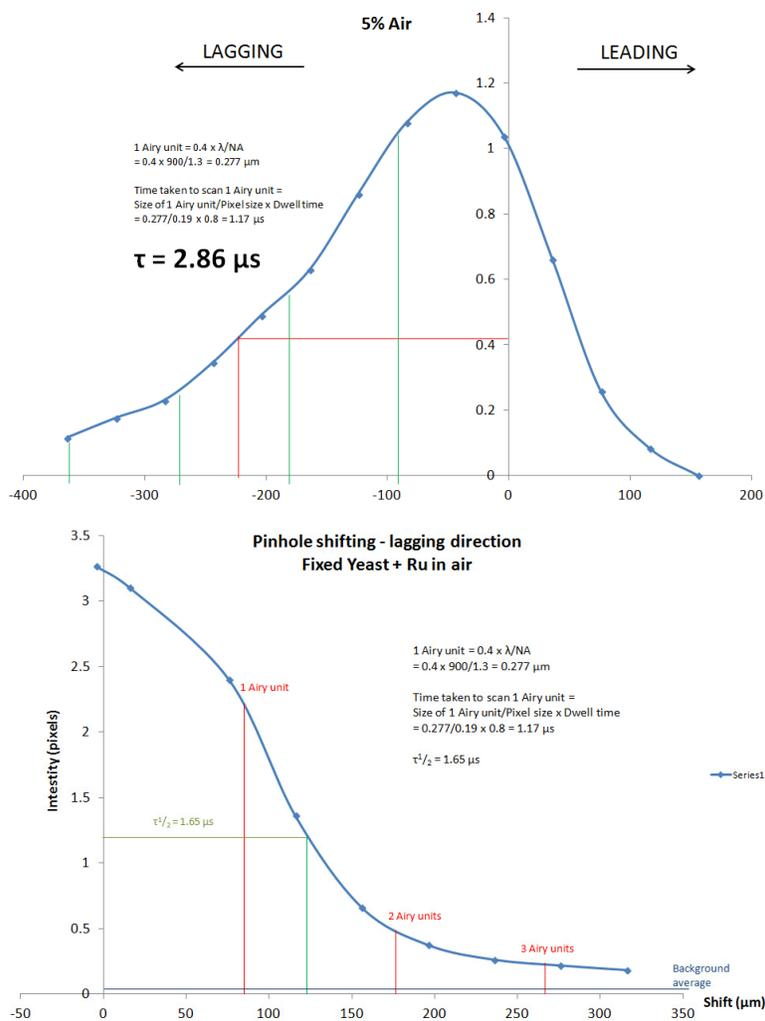
Fig. 2. Two examples of calculations of phosphorescence lifetime measurements from experiments with Ru nanoparticles in suspension or after electroporation into ethanol-fixed *Schizosaccharomyces pombe* that used the pinhole shifting method of Ramshesh and Lemasters.<sup>51</sup>
