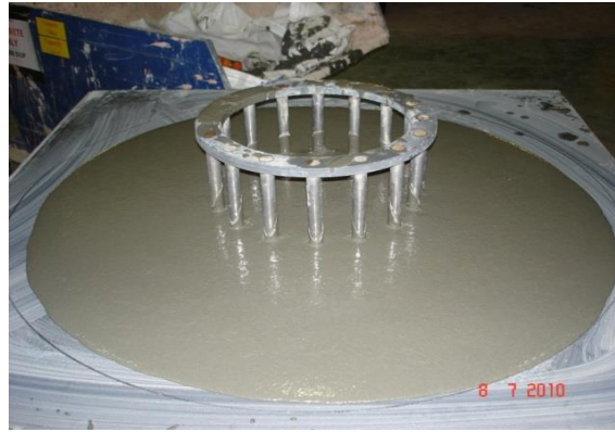
Figure 4.18: Flow and passing ability of SCUHPFRC Mix 8
