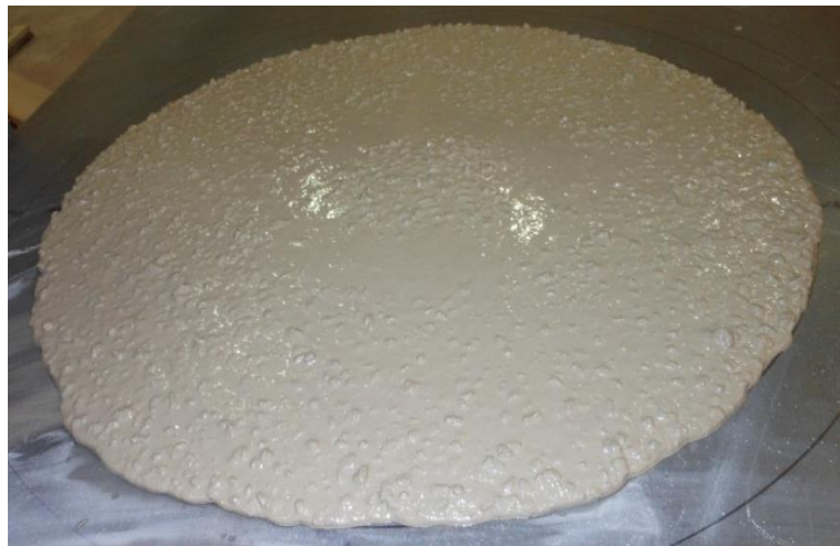
Figure 4.3: Horizontal spread of SCC Mix 2
