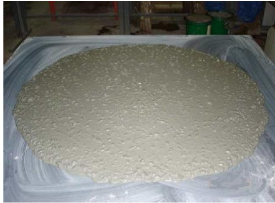
Figure 4.6: Horizontal spread of SCC Mix 6
