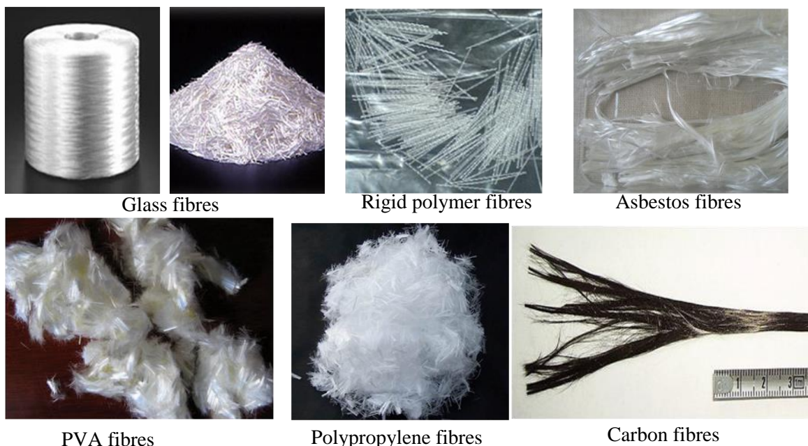
Figure 2.20: Different type of fibres used in concrete reinforcement
