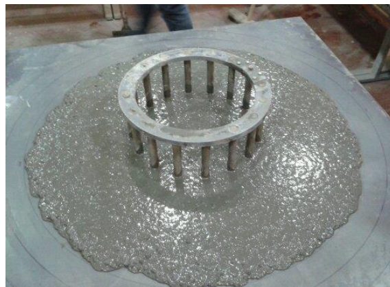
Figure 4.9: Flow and passing ability of Mix 5 (left) and Mix 6 (right)
