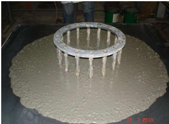
Figure 4.8: Flow and passing ability of SCC Mix 4
