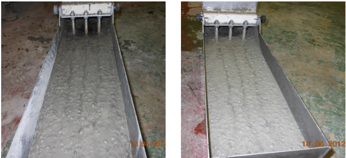
Figure 4.12: Flow and passing ability of SCC Mix 1 (left) and Mix 2 (right)
