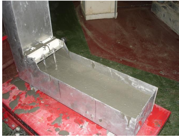
Figure 4.20: Flow and passing ability of SCUHPFRC (Mix 8)
