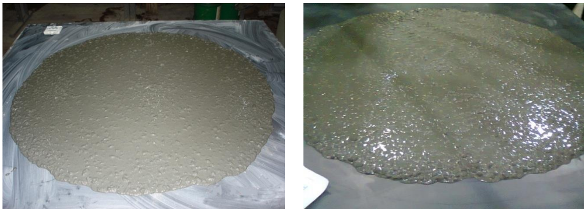
Figure 4.5: Horizontal spread of SCC Mix 4 (left) and Mix 5 (right)
