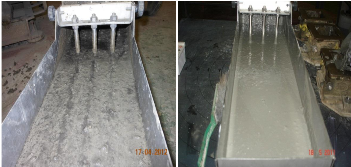
Figure 4.13: Flow and passing ability of SCC Mix 3 (left) and Mix 4 (right)
