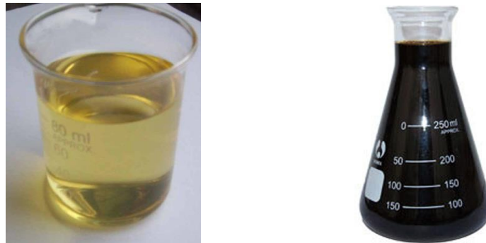
Figure 2.16: Polycarboxylate-based super-plasticiser (left) and sulfanate-based super-plasticiser (right)
