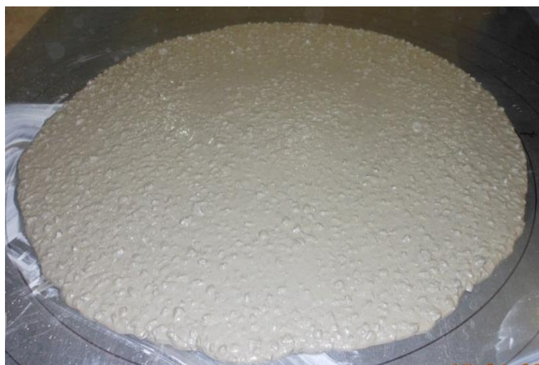
Figure 4.4: Horizontal spread of SCC Mix 3
