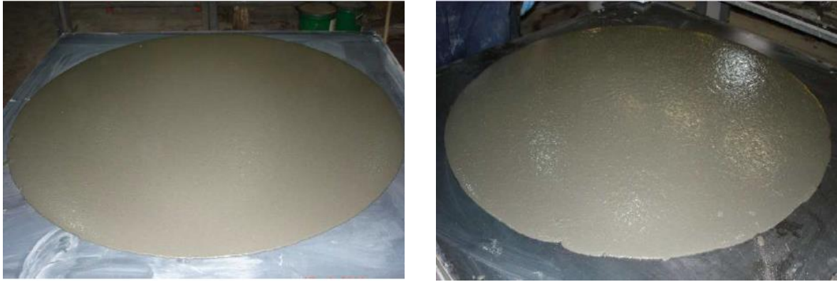
Figure 4.15: Horizontal spread of SCUHPC Mix 7 (left) and SCUHPFRC Mix 8 (right)
