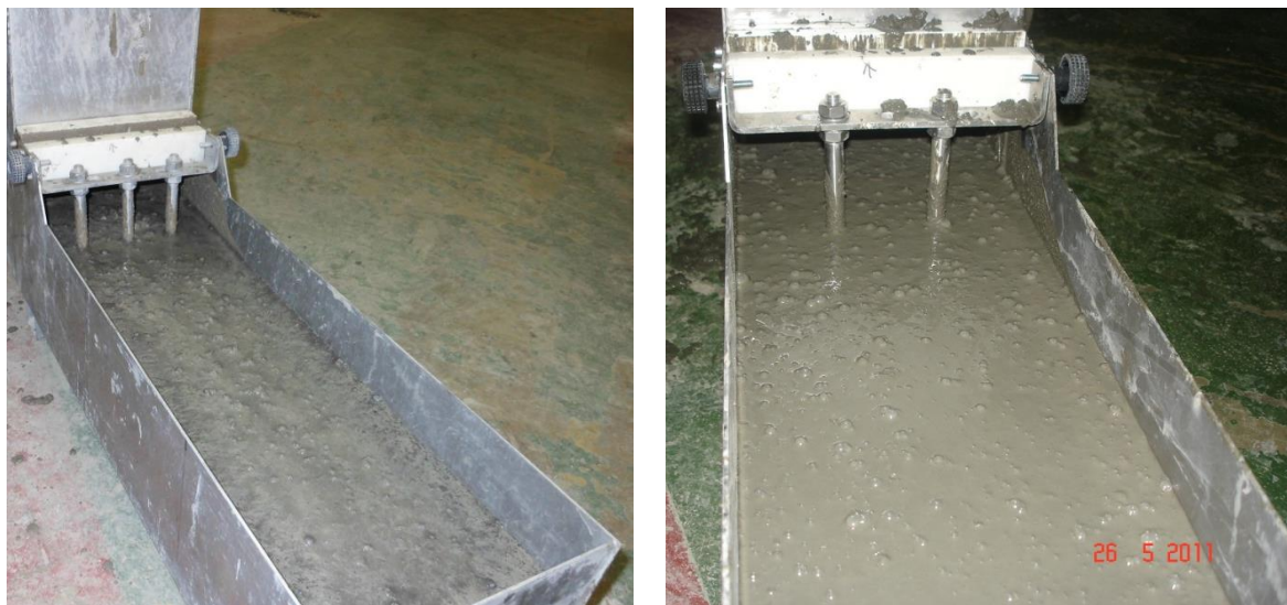
Figure 4.14: Flow and passing ability of SCC Mix 5 (left) and Mix 6 (right)
