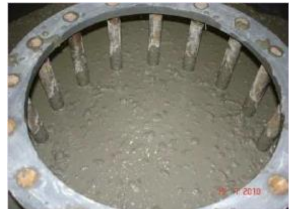
Figure 4.8: Flow and passing ability of SCC Mix 4
