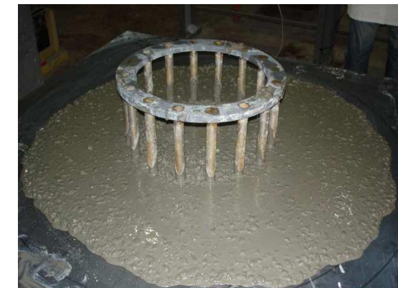
Figure 4.9: Flow and passing ability of Mix 5 (left) and Mix 6 (right)
