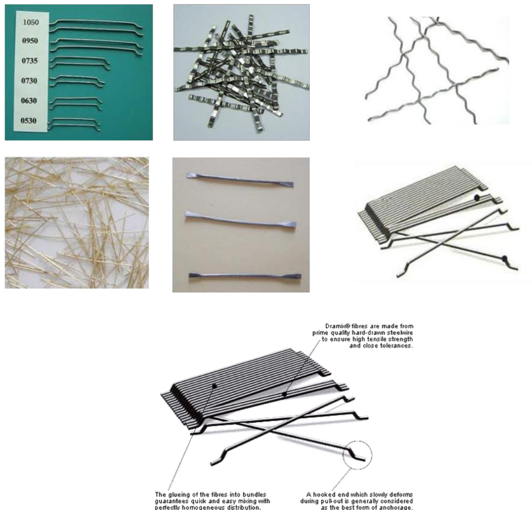
Figure 2.23: Different types of steel fibres used in reinforced concrete
