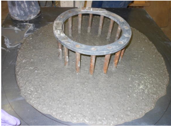
Figure 4.7: Flow and passing ability of SCC Mix 2 (left) and Mix 3 (right)
