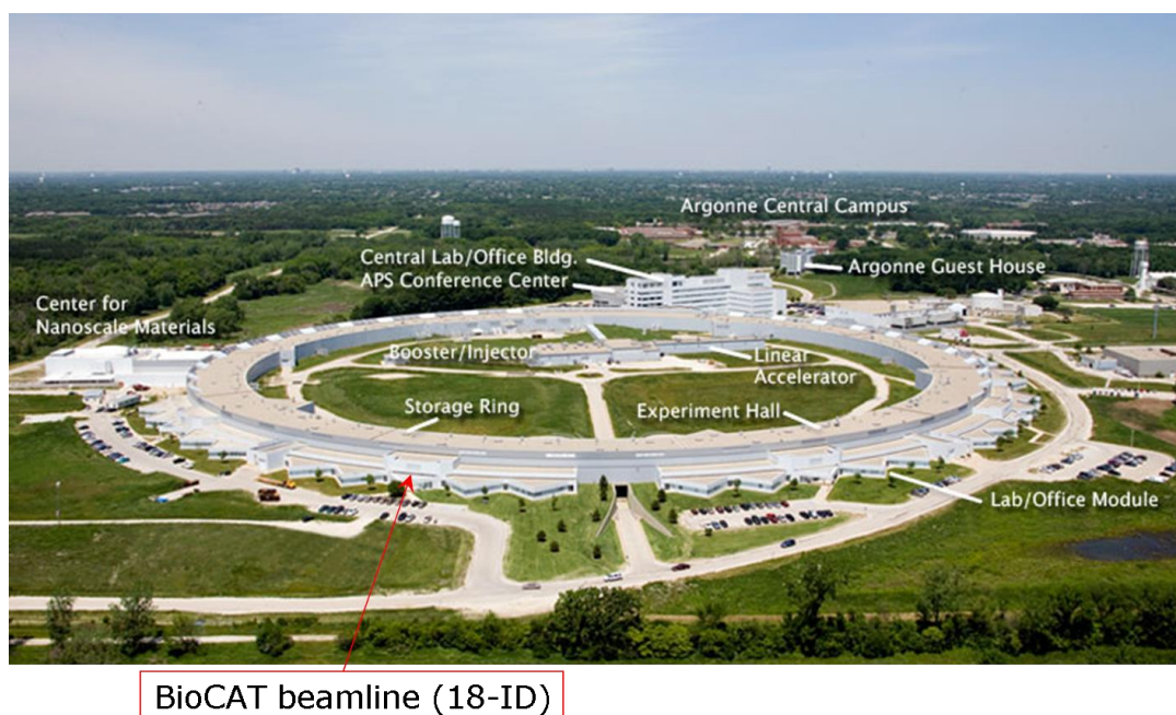
Figure 5.4 Aerial view of APS (from www.aps.anl.gov/About/APS_Overview , as of August 2013). The principle components of the synchrotron are labelled. The position of the BioCAT beam line used for the X-ray data collection portion of this work is indicated by the red arrow. For an idea of scale, cars can be seen on the photo and the circumference of the electron storage ring contained within the circular component of the building is 1104 m.
