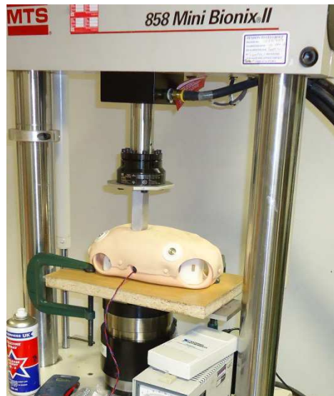
Figure 4-1: MTS 858 machine experimental set up to establish the compression stiffness and the maximum achievable compression depth of the modified manikin chest
