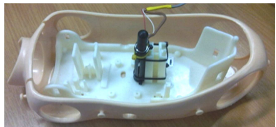
Figure 3-3: Laerdal® ALS Baby manikin instrumented with linear potentiometer
