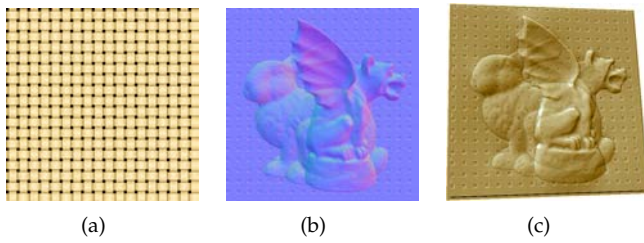
Fig. 24: Bas-relief modeling using an image and two 3D models: (a) a texture; (b) a composite normal image; and (c) the resulting bas-relief.
