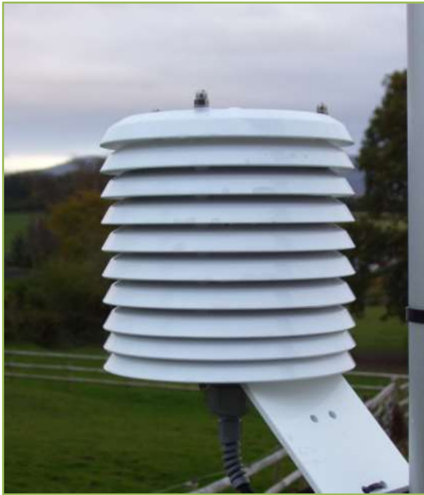
Figure 3.10 – Photograph of the installed solar shield which houses the combined temperature and relative humidity probe.
