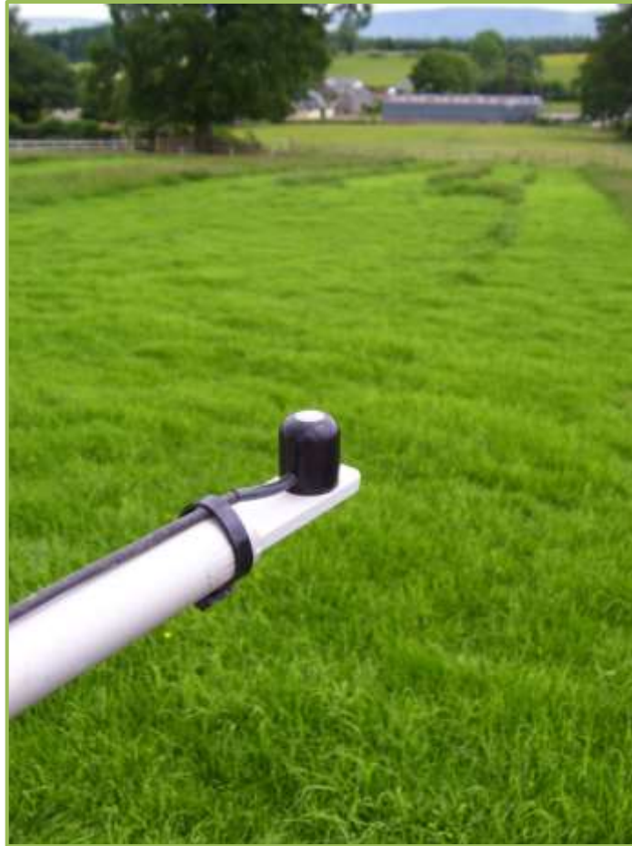
Figure 3.9 – Photograph of the installed silicon-cell pyranometer used to measure the short-wave radiation.
