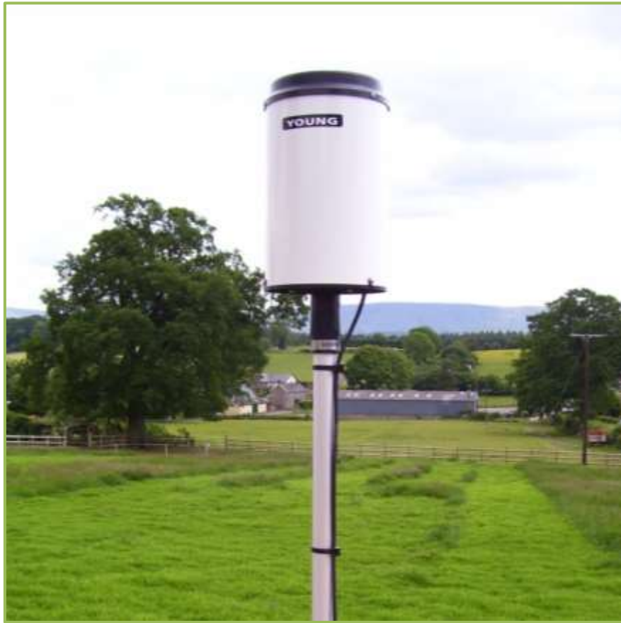
Figure 3.12 – Photograph of the installed tipping bucket rain gauge.
