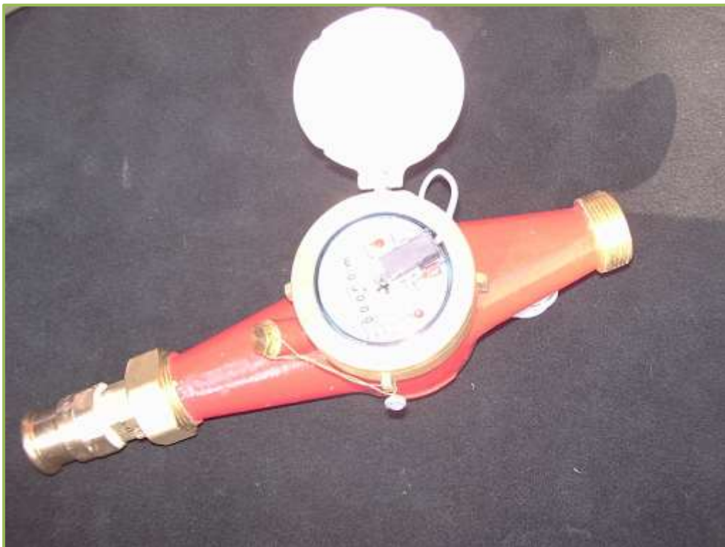
Figure 3.14 – Photograph of the Metron flow meter prior to installation.
