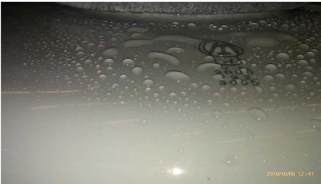
(c) Insulator surface newly Nanocoated (HC4)
