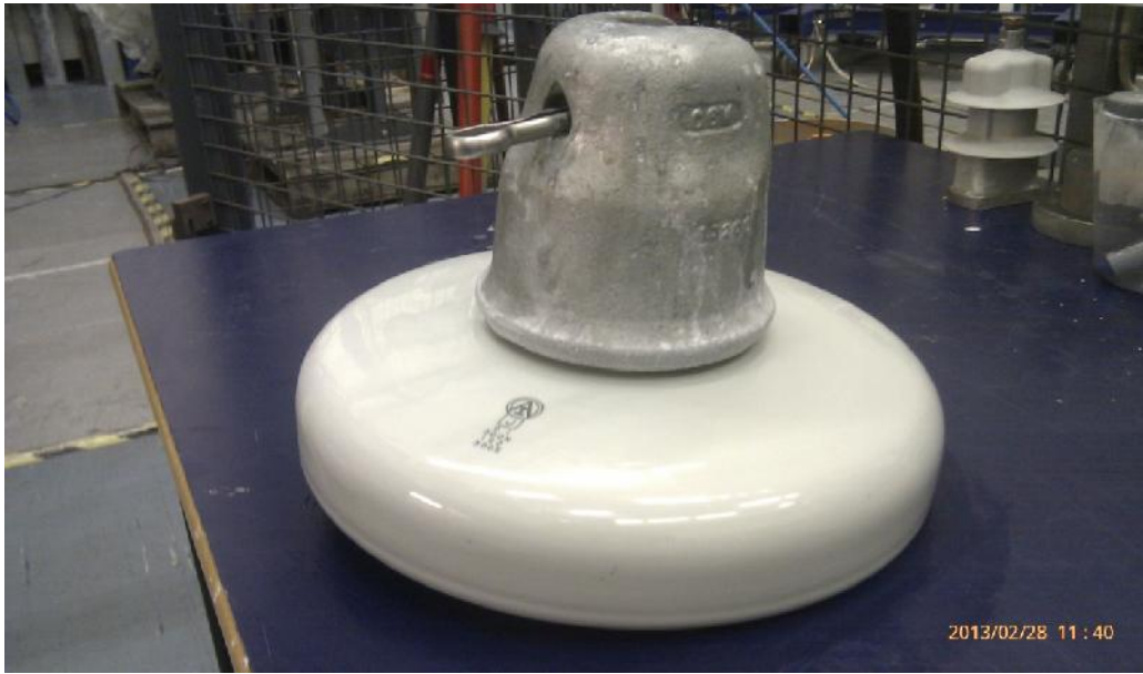
(a) Nanocoated insulator
