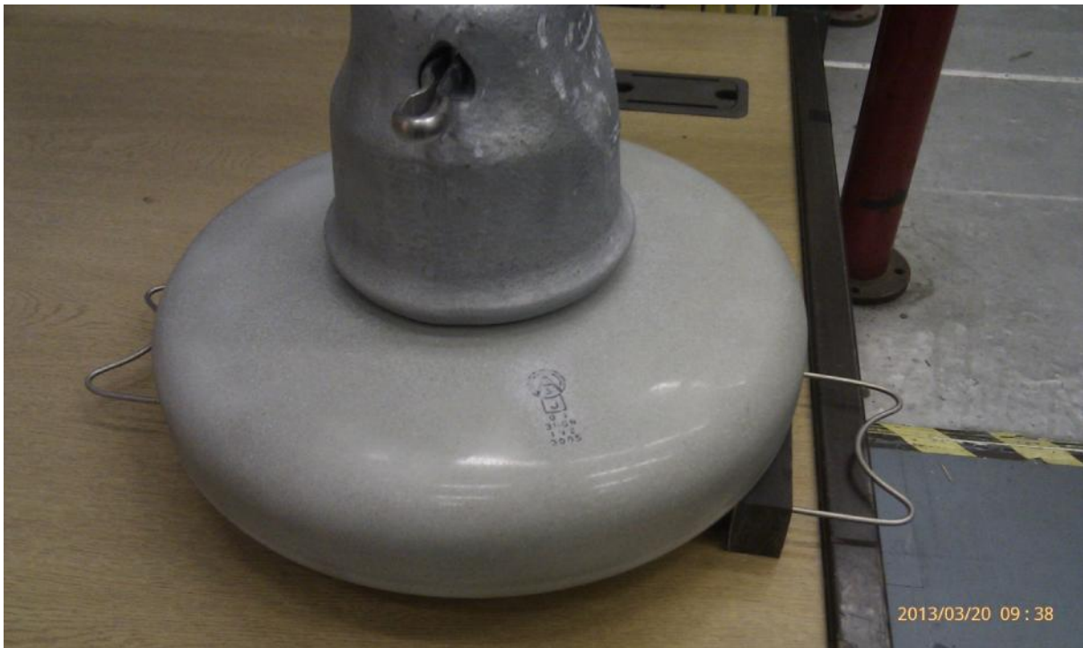
Figure 4.17: Nanocoated insulator after sandblast exposure
