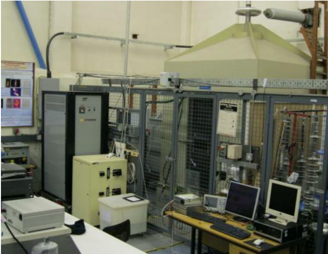
(b) Fog chamber in the high voltage laboratory (Cardiff University)
