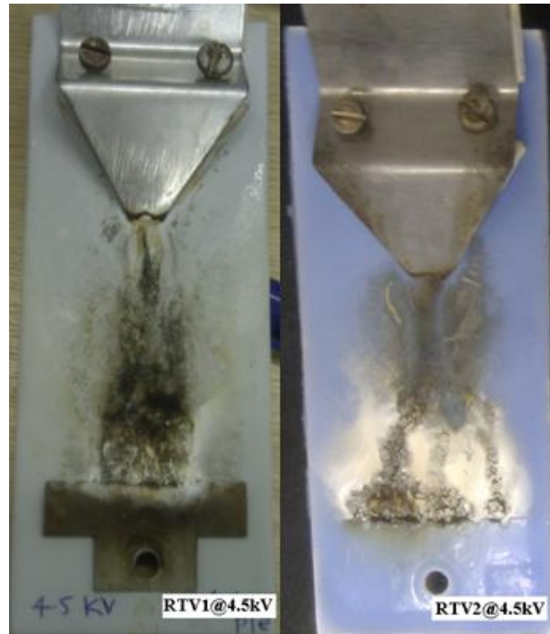
Figure 5.7: Photos of RTV1 and RTV2 tested at 4.5 kV for 6 hours
