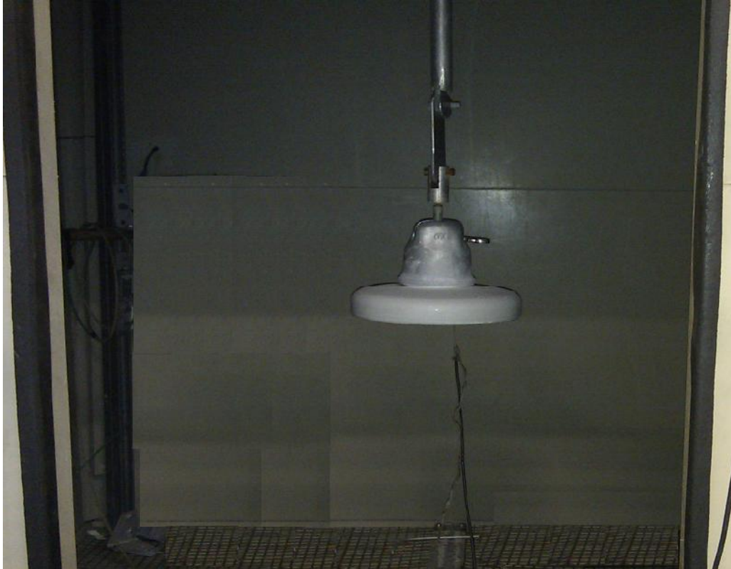
Figure 4.3: Insulator placed in the fog chamber
