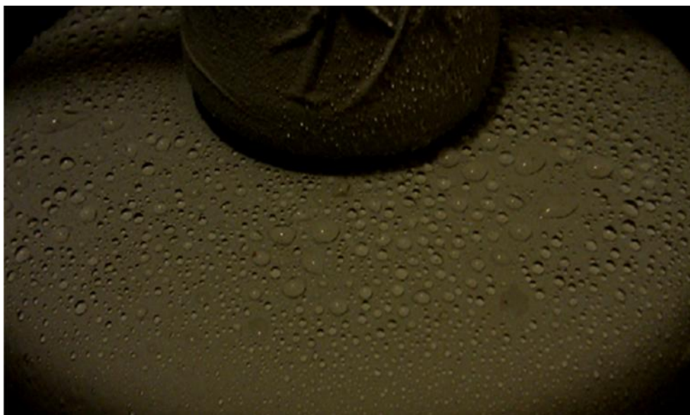
(a) Surface newly coated with RTV1 (HC1)
