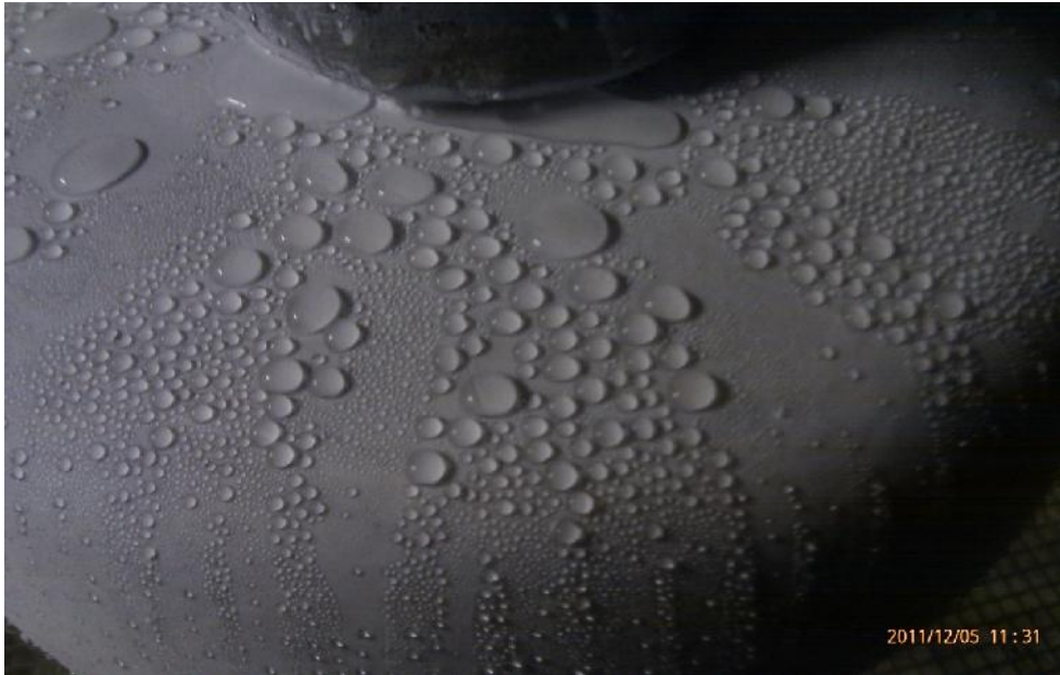
(b) RTV1 coating after 1hour wet test in the fog chamber (HC3)
