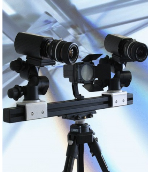
Figure 2.8 A typical 3D-DIC stereo-vision system setup 84
