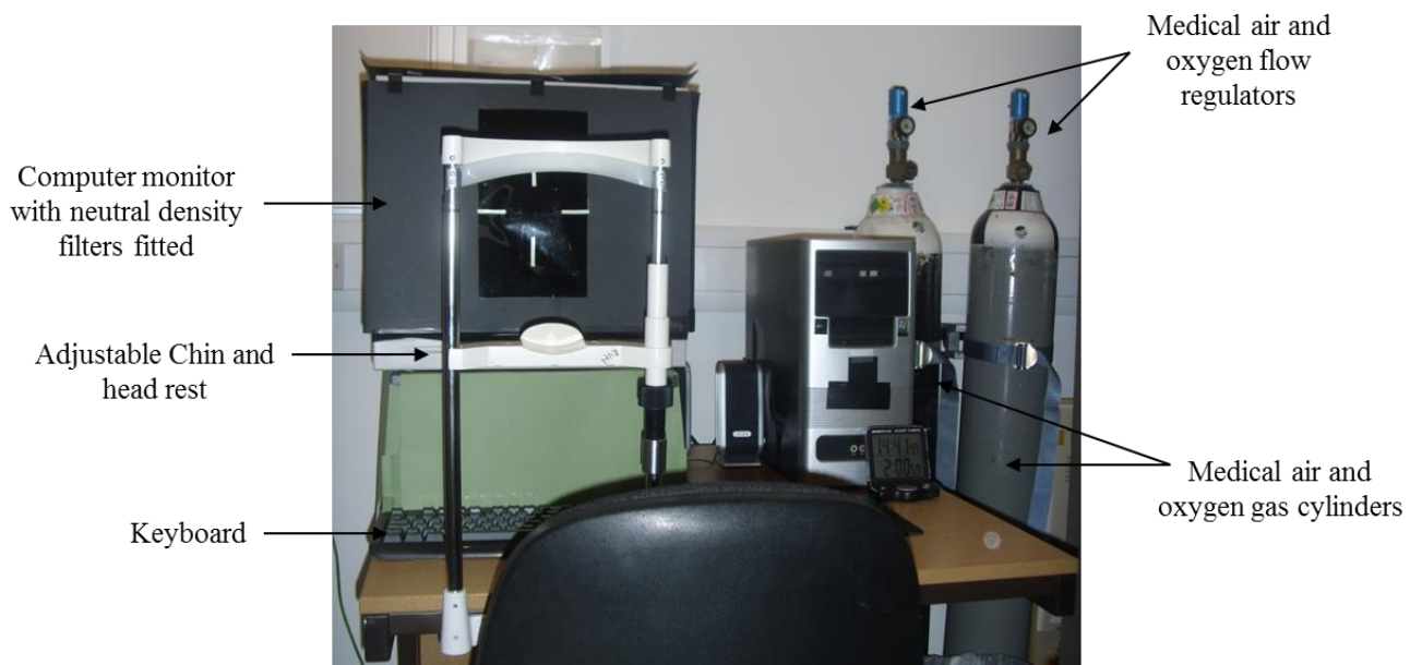
Figure 4.4 Photograph showing the set-up of equipment for testing dark adaptation whilst inspiring medical air or oxygen.
