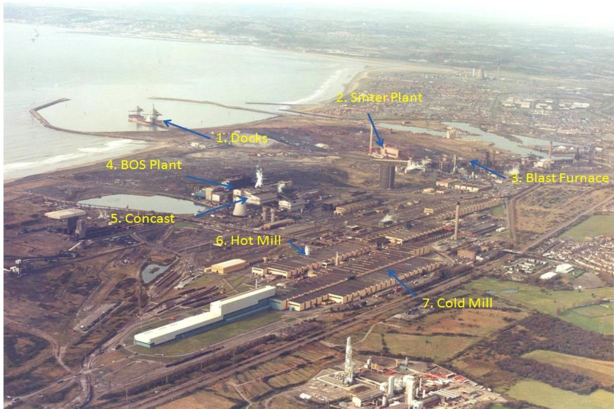
**Figure 4.8** Aerial view of the Port Talbot integrated steelworks with different various plant buildings labelled [102]
