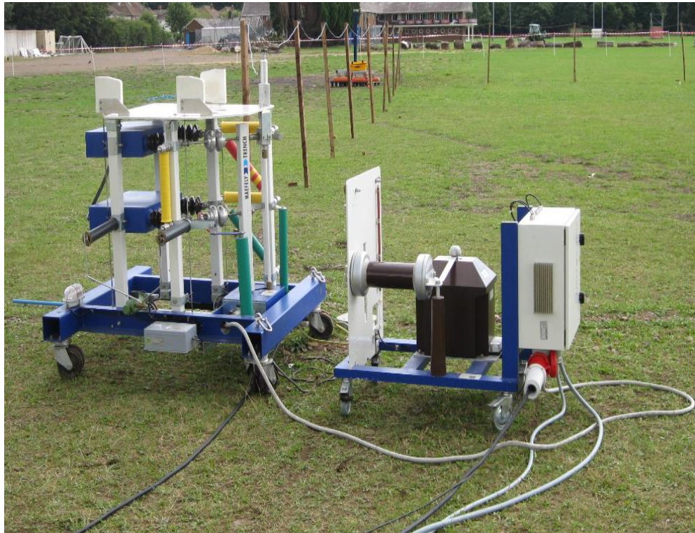
Figure 7.7: High current impulse generator at the field site
