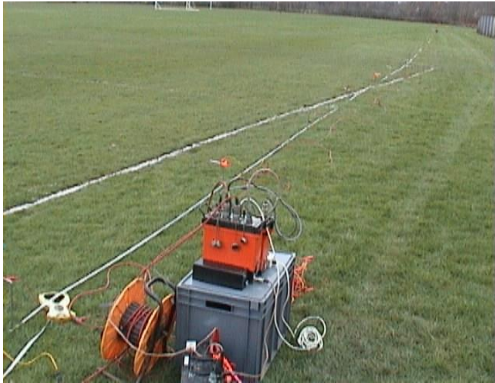
Figure 3.9: Test set-up for the ABEM/LUND imaging system
