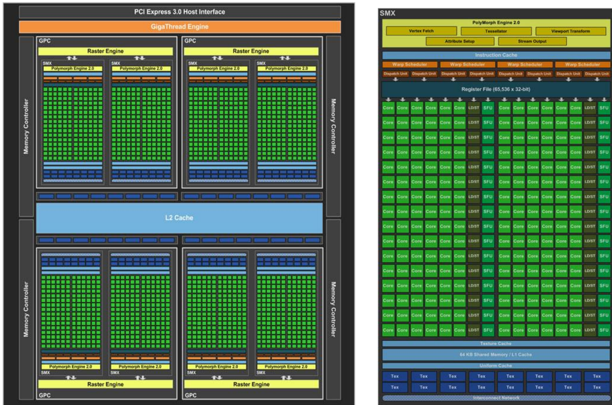
Figure 2-1: The GK104 (Kepler line) chip architecture. Image courtesy of NVIDIA
