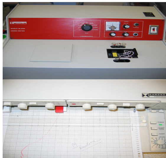
Figure 2.2: Chronolog platelet aggregometer used in our study to quantify platelet aggregation.
