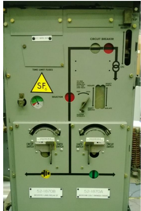
Figure 7.5: RMU positive lightning impulse gas insulation test position for ring switch.
