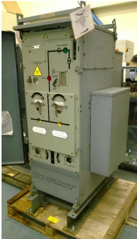
Figure 7.1: A Lucy SCRMU(M) ring main unit.
