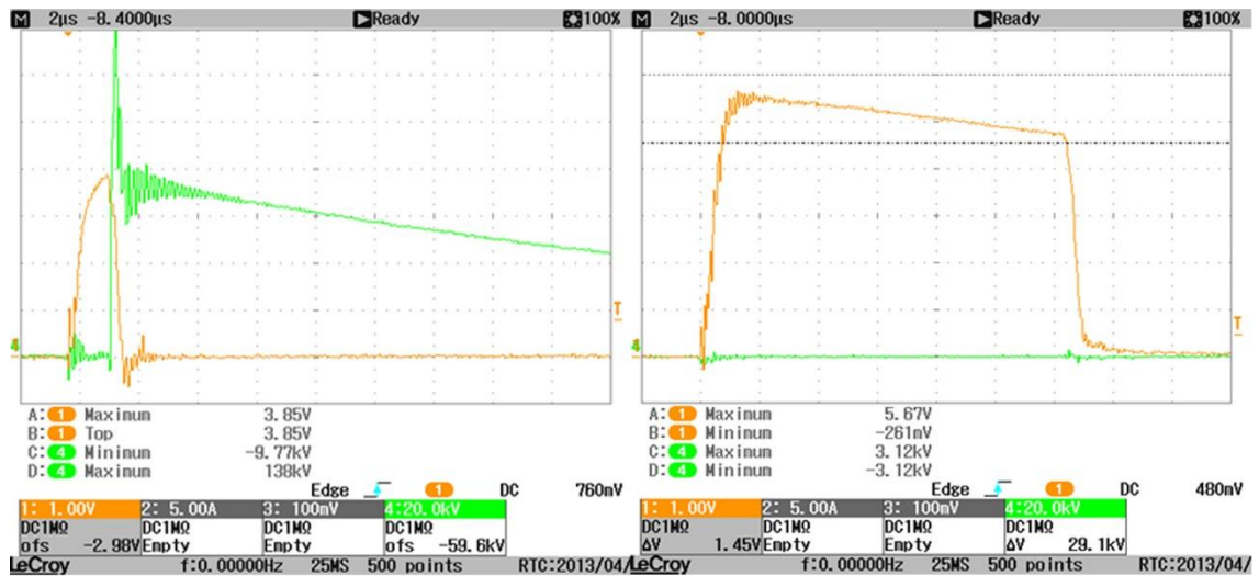
Figure 4.16: Applied LI to the Ringmaster 20%-80% CF 3 I-CO 2 switch disconnector – short time to breakdown
