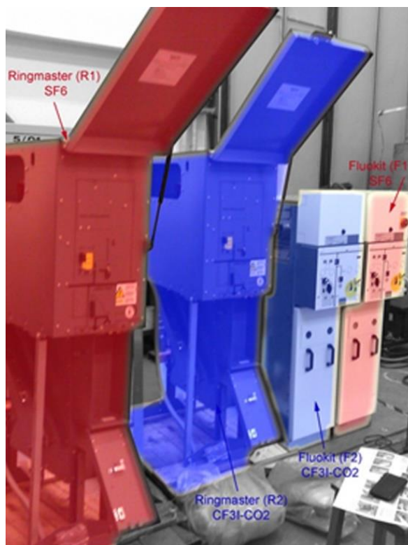
Figure 4.6: Ringmaster SE6 and Fluokit M24+ switch disconnectors used for testing red indicates SF 6 gas filled devices, blue indicates CF 3 I-CO 2 gas filled devices.
