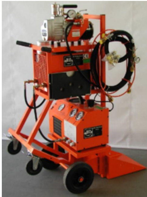
Figure 4.8: Dilo mini series complete with vacuum pump, filter, compressor and vacuum compressor for vacuuming, gassing and de-gassing switchgear [78].
