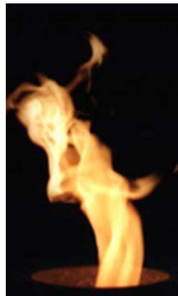
Figure 18: Visualisations of the PVC (a) its helical nature (b) with axial injection into a premixed flame adapted from Fick (1998)
