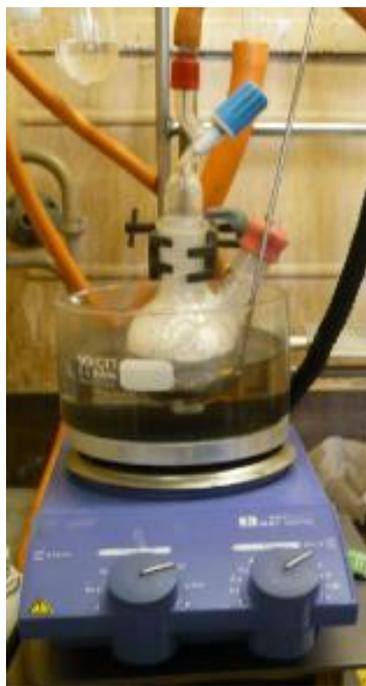
**Figure 2.1 Vacuum incipient wetness experimental set-up**
