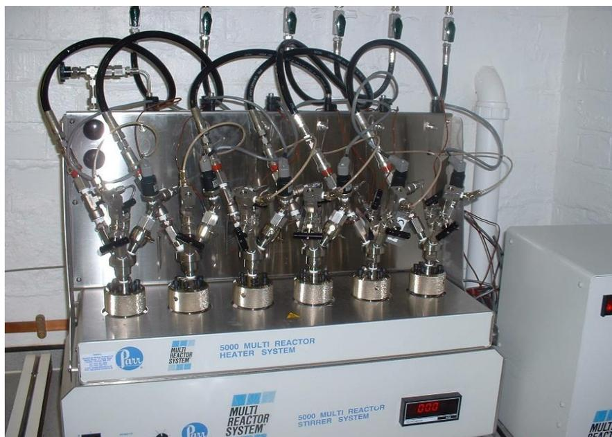
**Figure 2.7 Multi reactor system and control box.**
