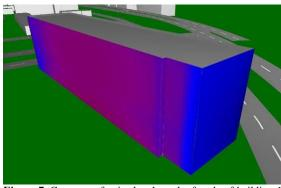
**Figure 7.** Contours of noise levels at the facade of building 1 in position A. Contours represent levels from 69 dB(A) in the purple zone to 79 dB(A) in the blue zone.
