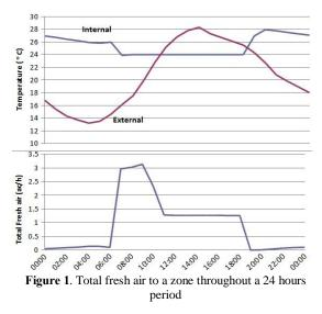
In addition to this standard modelled window opening pattern the opening percentage is adjusted so that the acoustic insulation of the facade at each window is not reduced to a level where the noise ingress exceeds a set tolerated level. This is done until windows are at maximum opening percentage or fully closed.
