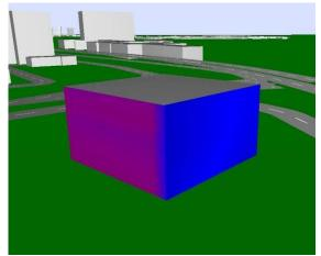
**Figure 9.** Contours of noise levels at the facade of building 2 in position A. Contours represent levels from 70 dB(A) in the purple zone to 77 dB(A) in the blue zone.
