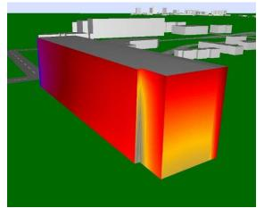
**Figure 8.** Contours of noise levels at the facade of building 1 in position A. Contours representing change in levels from 54 dB(A) in the yellow zone to 75 dB(A) in the blue zone.
