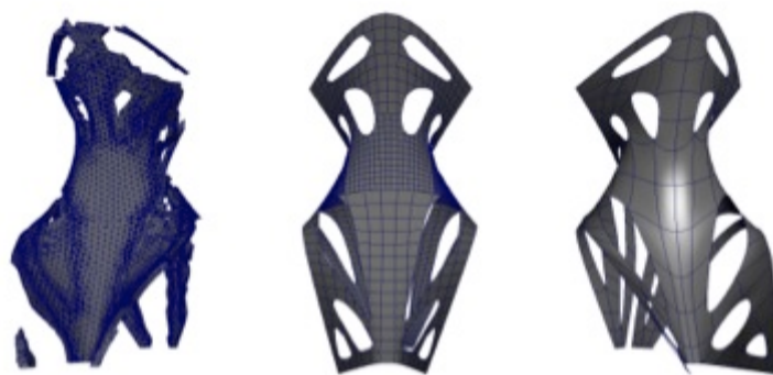
Figure 3: Left to Right : High resolution mesh FEM mesh ~50000 vertices ; multi-patch, medium resolution mesh ~6200 vertices ; low resolution, predominantly-quad, mesh ~ 275 vertices;
