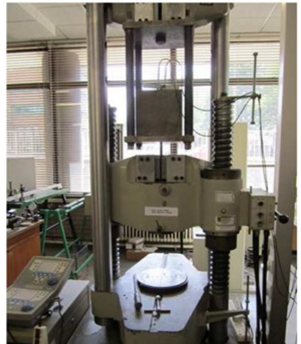
Figure 3.9: Pull-out test arrangement
